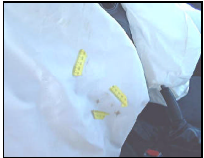
Figure 7. Driver's air bag contact evidence.
