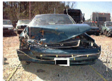
Figure 2. Frontal damage to the Subaru Legacy.
