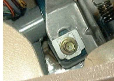
Figure 6. Left shear capsule displacement.
