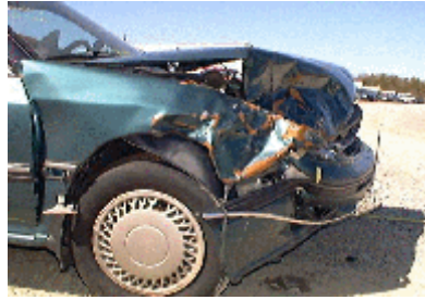
Figure 3. Profile view documenting the extent of frontal crush.
