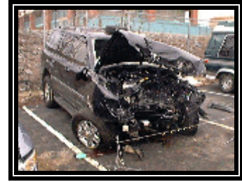
Figure 8. Frontal damage to the Lexus LX470.
