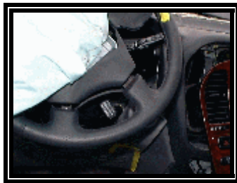
Figure 13. Right steering wheel spoke deflection.
