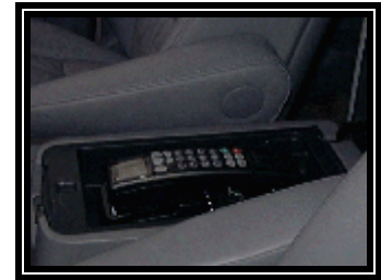
Figure 2. Hard wired cellular phone in the center console.
