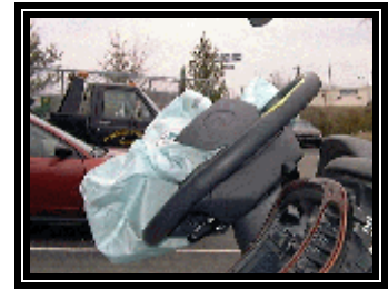
Figure 12. Deflection of the upper steering wheel rim.
