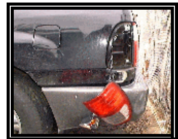
Figure 10. Secondary sideslap damage to the left rear quarter panel.
