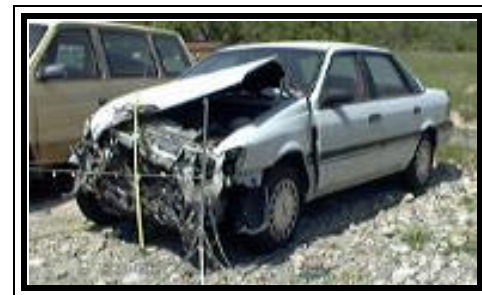
Figure 5. Frontal damage to the 1988 Ford Tempo.
