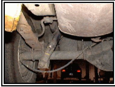
Figure 9. Dent to the lower unit of the right rear shock.
