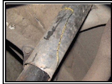
Figure 10. Dent and wipe mark to the upper shield of the shock absorber.
