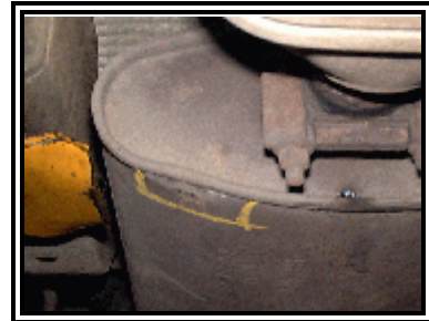
Figure 8. Abrasion to the muffler.
