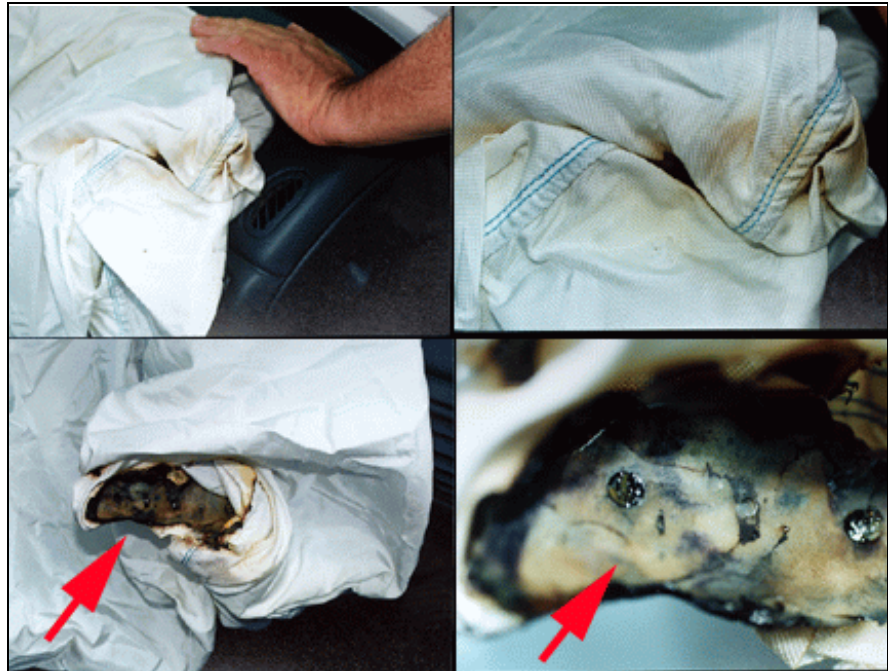
Figure 6. Passenger air bag. Shows exterior of air bag first, then the melted pieces of plastic found on the inside.
