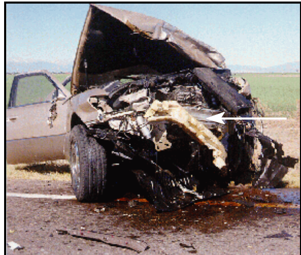
Figure 4: Vehicle #1's damaged frontal plane; Note: vertical bumper shift from impact with case vehicle (case photo #14)
