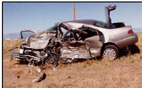
Figure 2: Case vehicle's frontal and left side direct damage; Note: post-crash location of left front wheel and upper/lower "A"-pillar (case photo #10)
