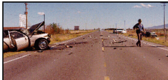
Figure 1: Case vehicle's southbound travel path showing absence of pre-impact braking marks; Note: case vehicle off road to right of Trooper, vehicle #1 off road to left (case photo #01)
