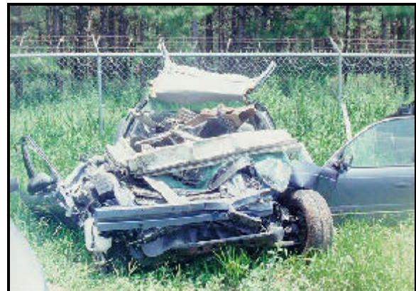
Figure 3: Front of case vehicle, with A- and B-pillars cut, roof peeled back and debris piled on (case photo #9)
