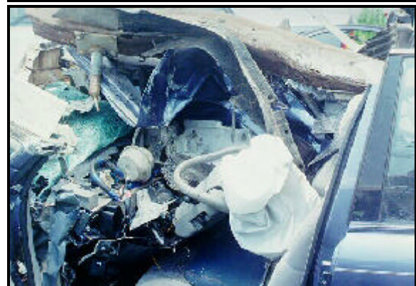
Figure 4: Case vehicle driver seat area; Note, deformed and intruded steering assembly and instrument panel (case photo #11)
