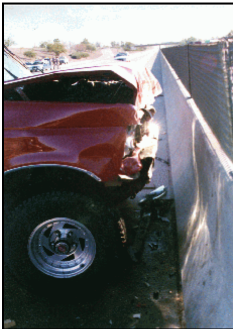
Figure 17. Exterior, Vehicle 4 (right side). Note the lack of contact to the barrier.
