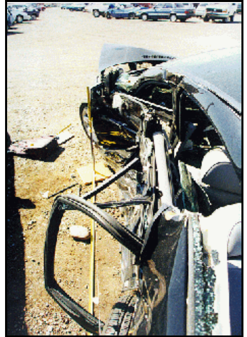
Figure 22. Left side of vehicle showing intruding components
