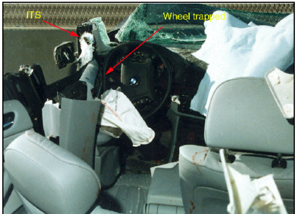
Figure 23. Shows ITS and left side air bag
