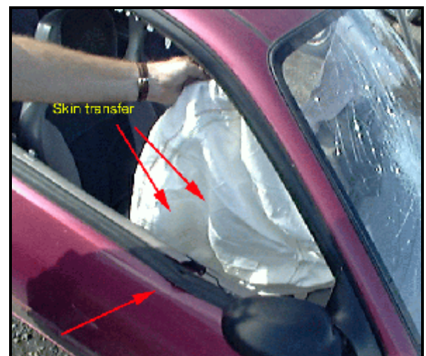
Figure 9. Interior, case vehicle—air bag / side glass frame interaction
