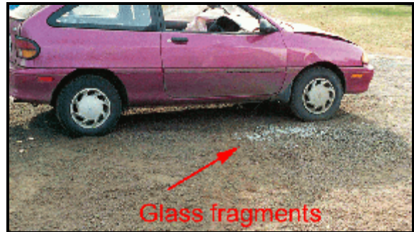
Figure 2. Side glass broken by front right occupant
