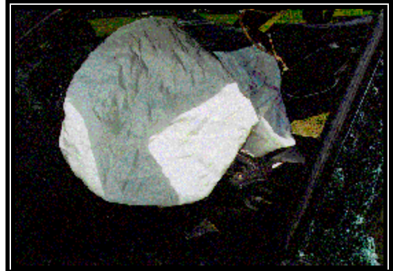
Figure 8: Driver air bag. Note, the steering wheel is rotated 180 degrees CCW.
