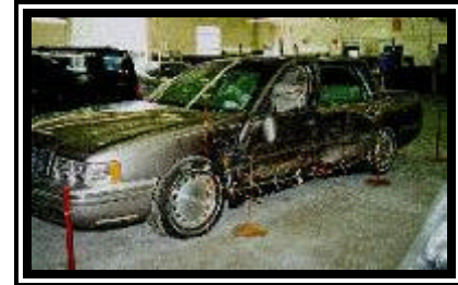
Figure 3. Left side damage to the 1997 Cadillac Deville.
