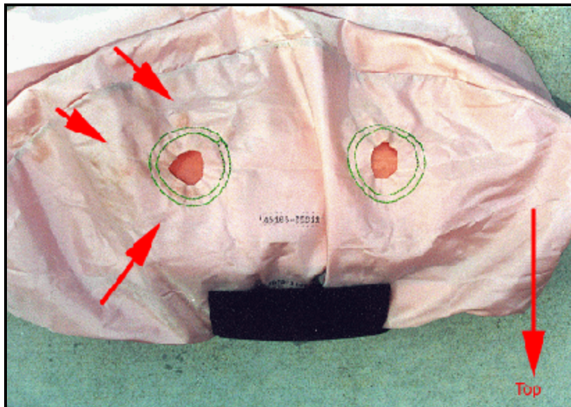
Figure 7. Back side of driver air bag—arrows indicate blood/saliva markings
