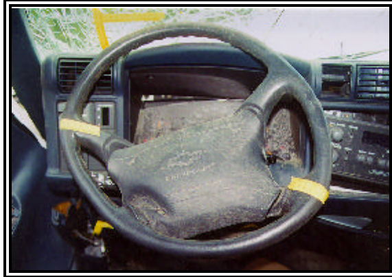
Figure 5: View of the steering wheel deformation.
