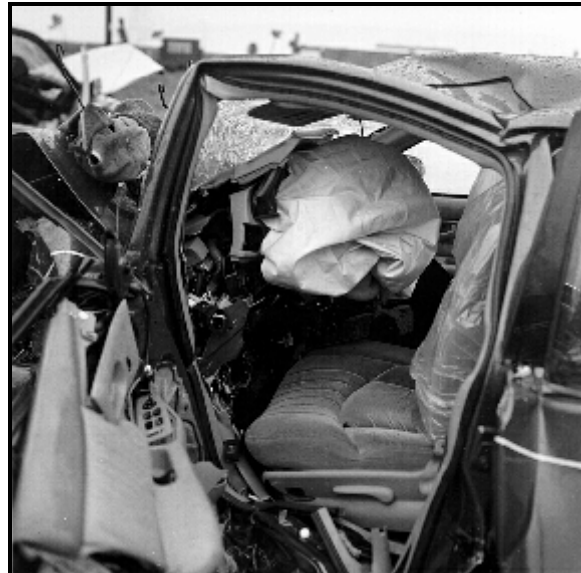
Figure 5: Case vehicle's driver seat area; Note: intruding components caused reduction of occupant space (case photo #12)
