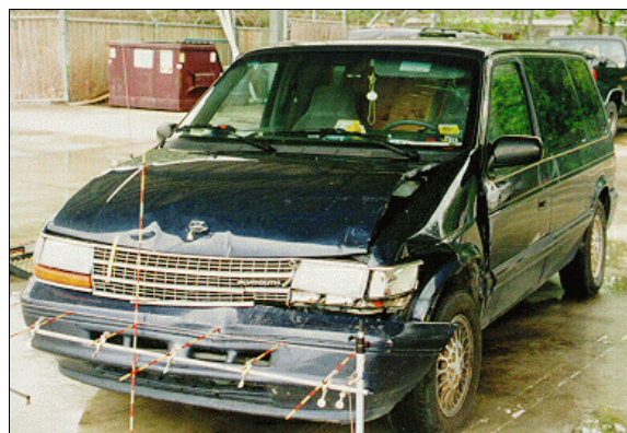
Figure 3: Case vehicle's frontal damage viewed from left of center; Note: damage from impact with back of Honda (case photo #11)
