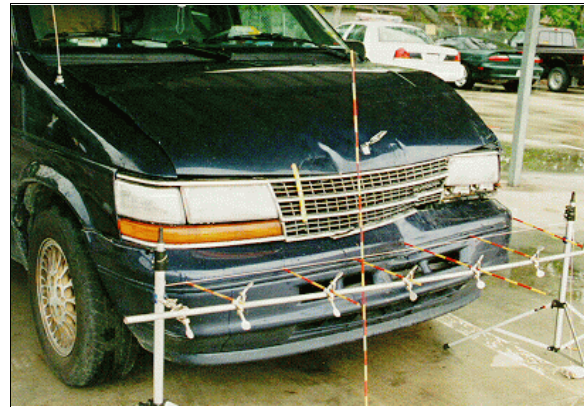
Figure 6: Case vehicle's frontal damage viewed from right of center (case photo #13)
