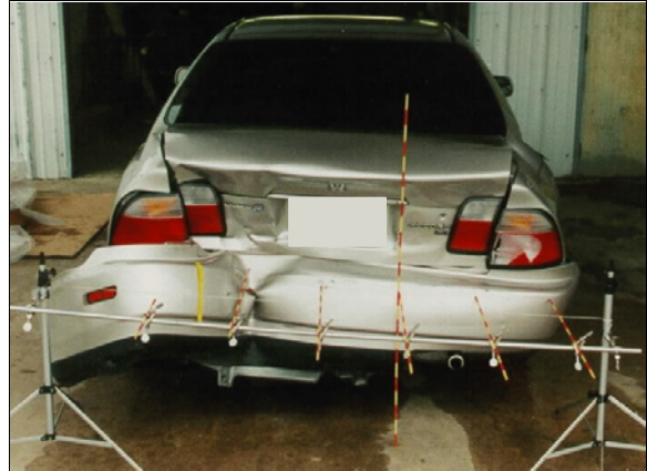
Figure 15: Honda's damaged back showing offset nature of crush profile; direct damage extends leftward from back right corner to yellow tape (case photo #56)
