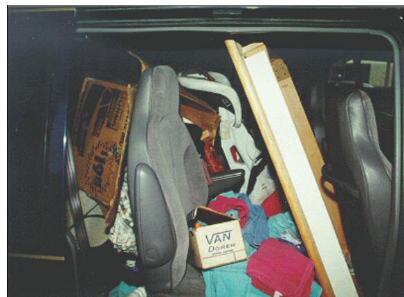
Figure 13: Case vehicle's second seating area viewed from sliding door showing excess cargo loaded behind front seats; Note: child safety seat stuffed between second left seat's seat back and table (case photo #53)
