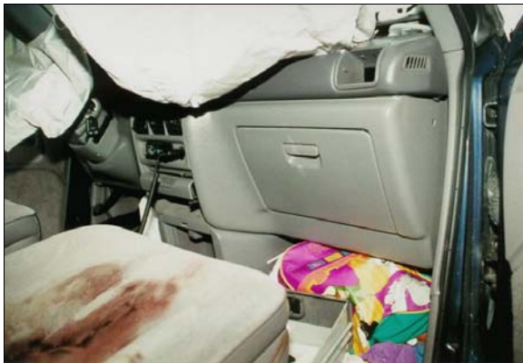
Figure 7: Case vehicle's front right seating area showing blood evidence on front right seat cushion, scuffs to glove box door, and blown out air vent in right instrument panel (case photo #32)
