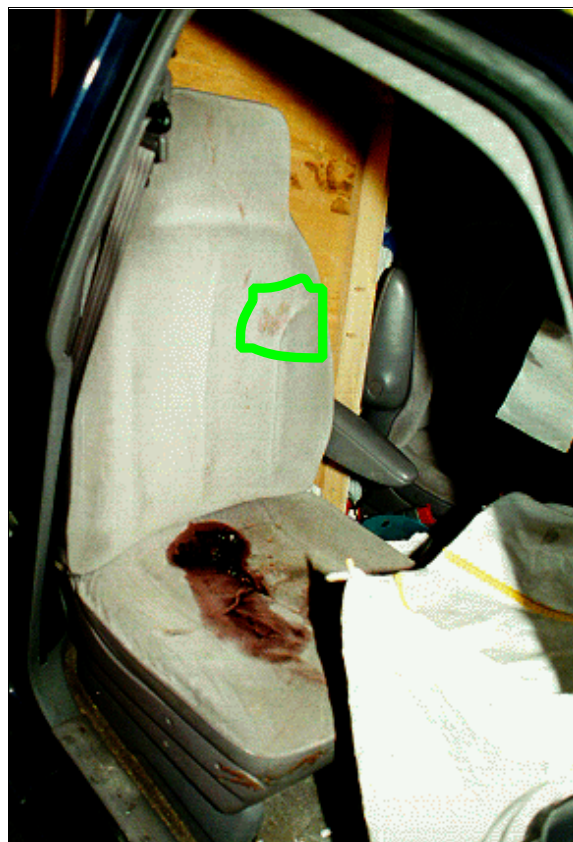
Figure 9: Case vehicle's front right seat showing pooled blood on seat cushion and head contact (i.e., outlined) to seat back (case photo #31)
