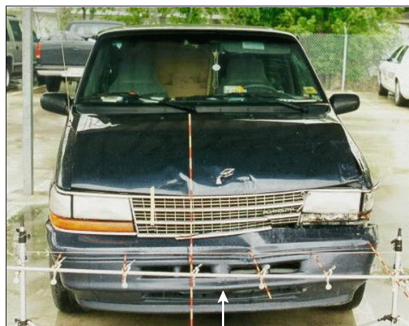
Figure 5: Case vehicle's frontal damage; Note: direct damage extends from front left corner rightward to yellow tape and slight imprint (arrow) from Honda's tailpipe (case photo #07)
