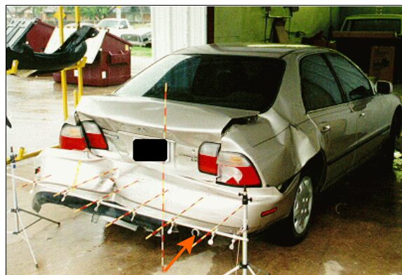
Figure 4: Deformation to back of Honda from impact with case vehicle; Note: impact offset toward right side and location (arrow) of tailpipe—see Figure 5 below (case photo #58)
