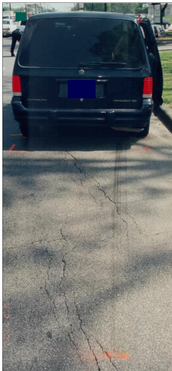
Figure 1: On-scene eastward view showing case vehicle's pre-crash trajectory and final rest position; Note: rightward yawing skid mark (case photo #63)
