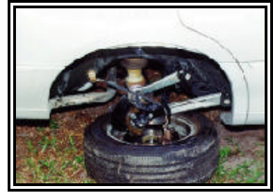
Figure 9. Displaced right rear wheel
