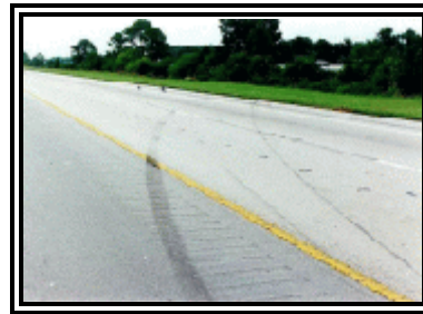
Figure 6. Tire marks showing path to final rest
