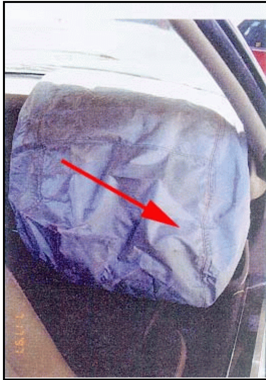
Figure 7. Passenger air bag. Arrow depicts likely contact between case occupant and air bag.
