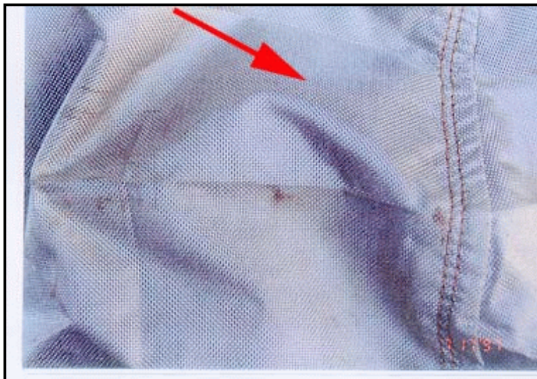
Figure 8. Close up of contact to air bag.
