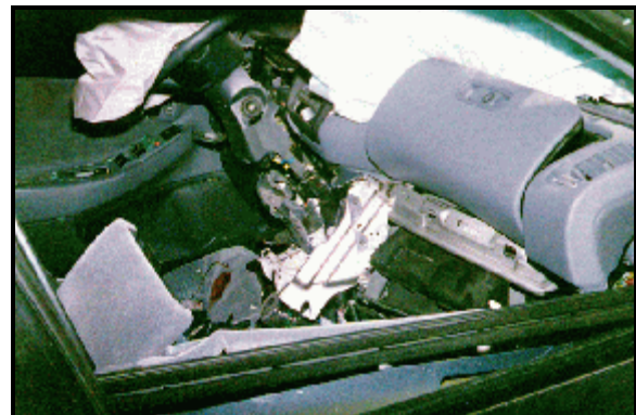
Figure 6: Case vehicle's post-impact interior; Note: rotation of instrument panel and position of the steering column (case photo #28)
