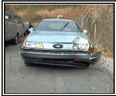
Figure 3. Frontal damage to the Ford Taurus.
