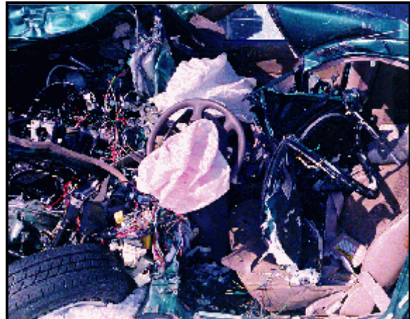
Figure 4: Case vehicle's interior damage; Note: left front door frame placed in driver's seat and position of steering wheel, possibly moved by extrication efforts (case photo #11)
