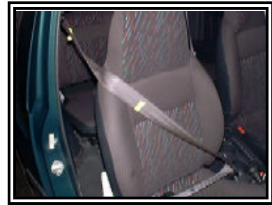
Figure 13. 3-point lap and shoulder belt system improperly worn by child passenger.
