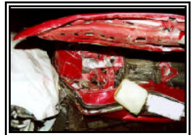
Figure 3. View showing damage across the frontal plane of the Cavalier
