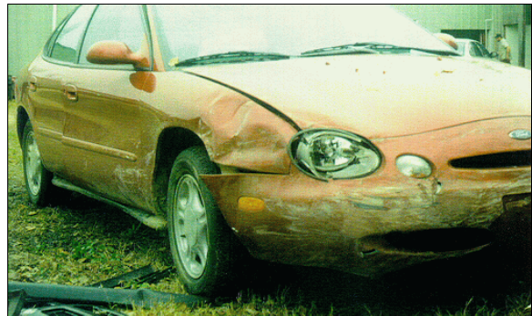
Figure 2: Minor deformation to case vehicle's front right bumper and right fender (case photo #02)
