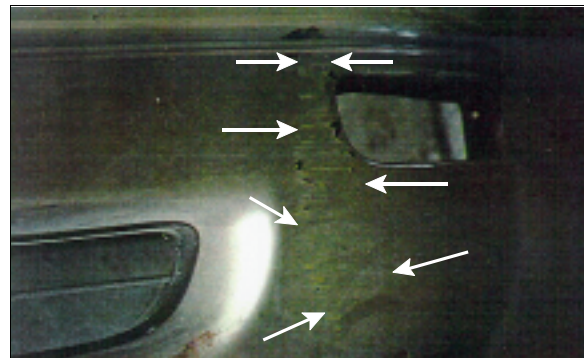
Figure 9: Close-up of vertically oriented direct damage at case vehicle's front left bumper; Note: contact came from shrub (case photo #21)
