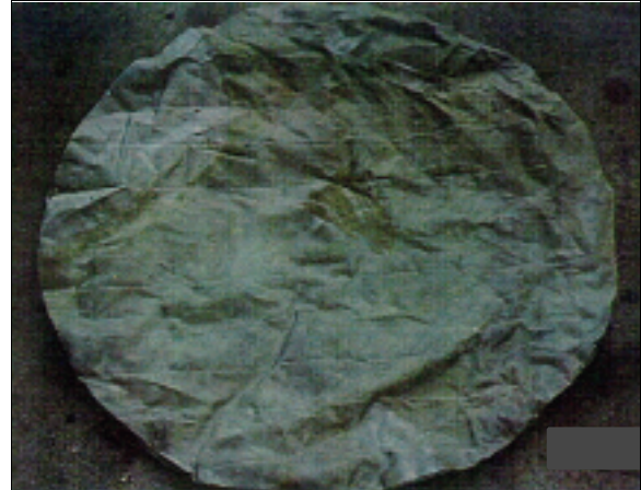
Figure 13: Case vehicle's removed (i.e., cut out) driver air bag showing evidence (i.e., bloodstain) of occupant contact (case photo #23)
