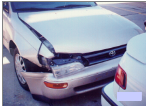
Figure 5: Case vehicle's damaged front showing damage to right hood, headlight assembly, and fender; Note: damage extends across entire front bumper (case photo #07)
