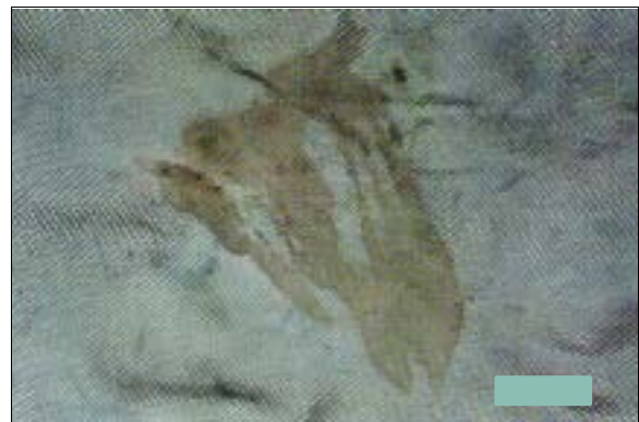
Figure 14: Close-up of occupant contact evidence (i.e., bloodstain) in center of case vehicle's driver air bag (case photo #24)
