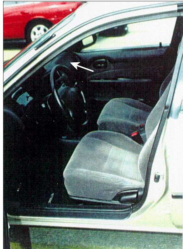
Figure 10: Case vehicle's front seating area, post repair, showing driver's steering wheel-mounted air bag module and mid instrument panel-mounted (arrow) front right air bag module (case photo #22)
