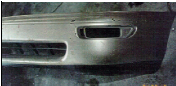
Figure 8: Case vehicle's damaged front bumper showing direct contact laterally across bumper and vertically at front left corner (case photo #20)
