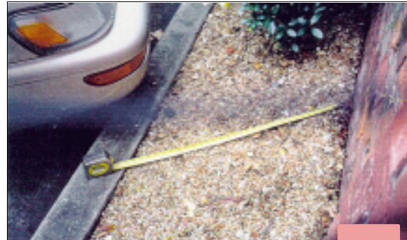
Figure 4: Distance between parking lot's curb and brick wall which enabled case vehicle's front to impact wall at approximately same time as right front tire struck curb (case photo #06)
