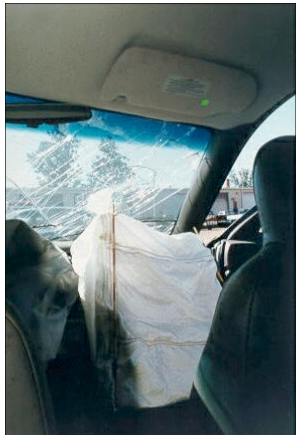
Figure 8: Case vehicle’s front right passenger seating area showing deployed front right passenger air bag, tow yard damage to right windshield’s glazing and either mucous spray or bag exhaust residue on front right sun visor (case photo #26)
