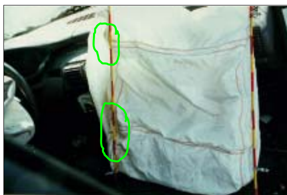
Figure 14: Case vehicle’s deployed front right air bag; Note: highlighted discolored areas (case photo #36)
