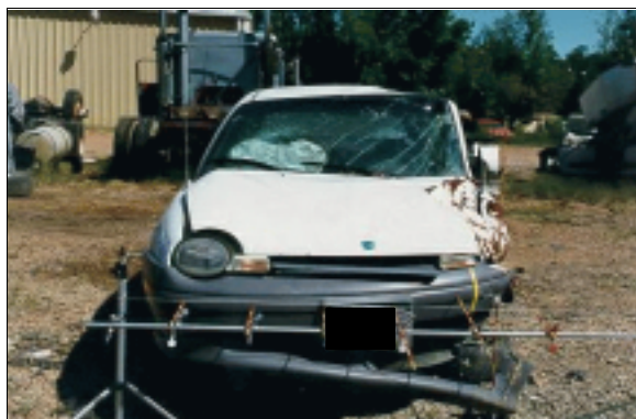
Figure 3: Case vehicle’s very narrow front left corner damage; Note: yellow tape marks rightward extend of direct damage (case photo #09)
