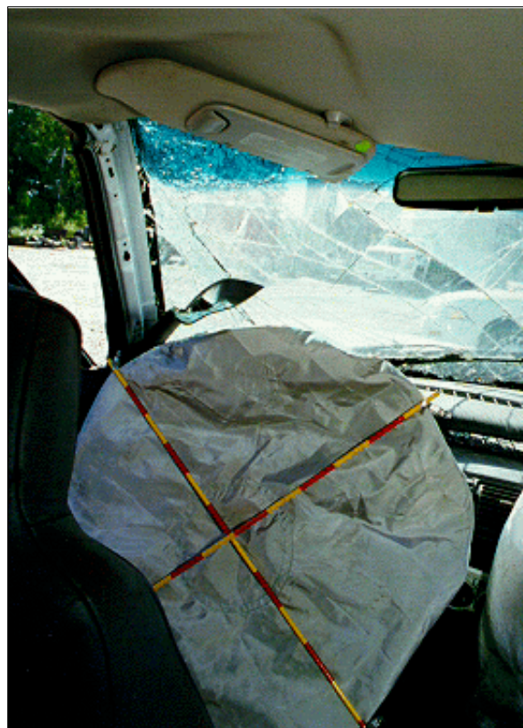
Figure 13: Vertical view of case vehicle's driver seating area and deployed air bag showing contact evidence near center of air bag; Note: intrusion to "A"-pillar and air bag exhaust residue on sun visor (case photo #23)
