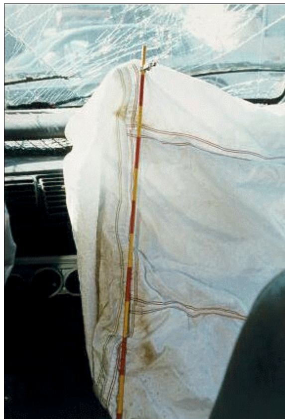
Figure 15: Close-up of case vehicle’s deployed front right passenger air bag showing bloody discoloration along left side surface (case photo #38)
