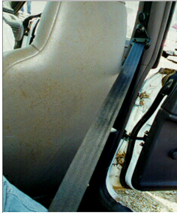
Figure 17: Vertical view of case vehicle's front right seat belt showing no apparent evidence (i.e., blood or loading) on webbing (case photo #40)
