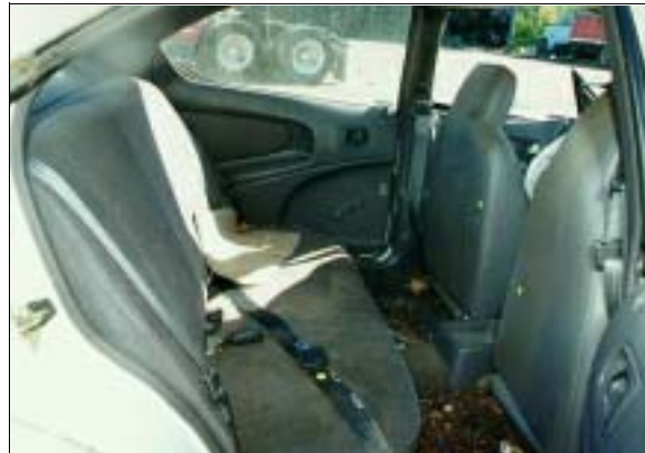
Figure 12: Case vehicle's back seating area; Note: deformed front seat backs from contact by back seat passengers (case photo #32a)
