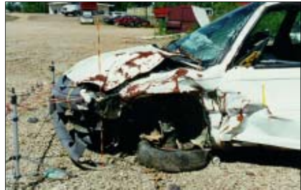
Figure 7: Case vehicle’s very narrow frontal impact showing deformation down left side; Note: yellow tape indicates length of direct contact (case photo #10)
