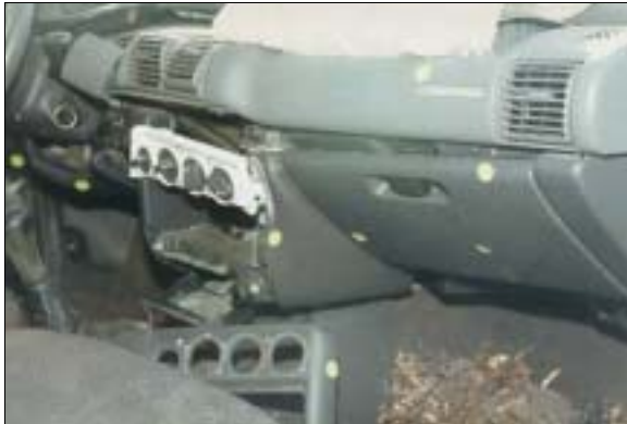
Figure 9: Case vehicle's instrument panel and glove box door showing deployed front right passenger's air bag and contact evidence around steering column, on center instrument panel and right glove box door (case photo #30)
