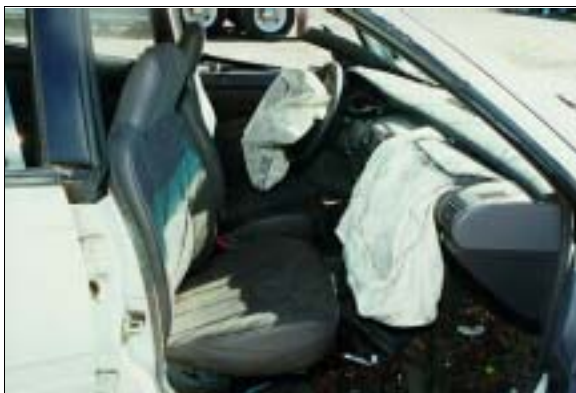
Figure 11: Case vehicle's front seating area showing deployed driver and front right passenger air bags; Note: both front seat backs deformed by passenger impacts from rear (case photo #32)
