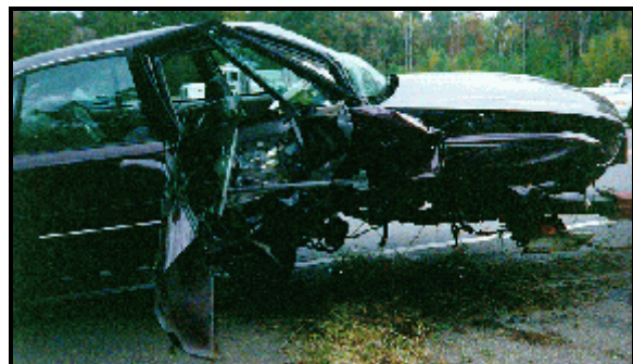
Figure 4: Case vehicle's undercarriage damage to right side; Note: right front wheel assembly and suspension under passenger's seat (case photo #07)
