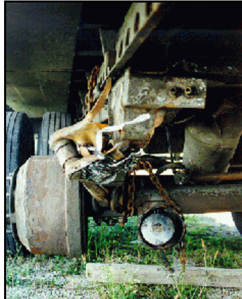
Figure 9: Close-up of vehicle #1 trailer's undercarriage showing struck right main spring and brake actuator (case photo #19)
