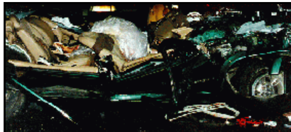
Figure 5: Right side of case vehicle after extrication; NOTE: outward deformation (case photo #12)
