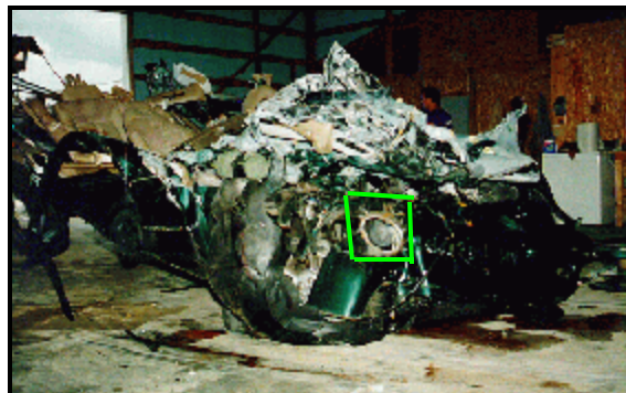
Figure 6: Angle view from front right of case vehicle; NOTE: V#1's brake actuator cover embedded into fender and right side components deformed outward (case photo #14)
