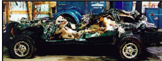
Figure 4: Left side of case vehicle after extrication; NOTE: inward deformation (case photo #07)
