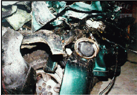
Figure 8: Close-up of vehicle #1 trailer's right brake actuator cover embedded into the case vehicle's right front fender (case photo #15)
