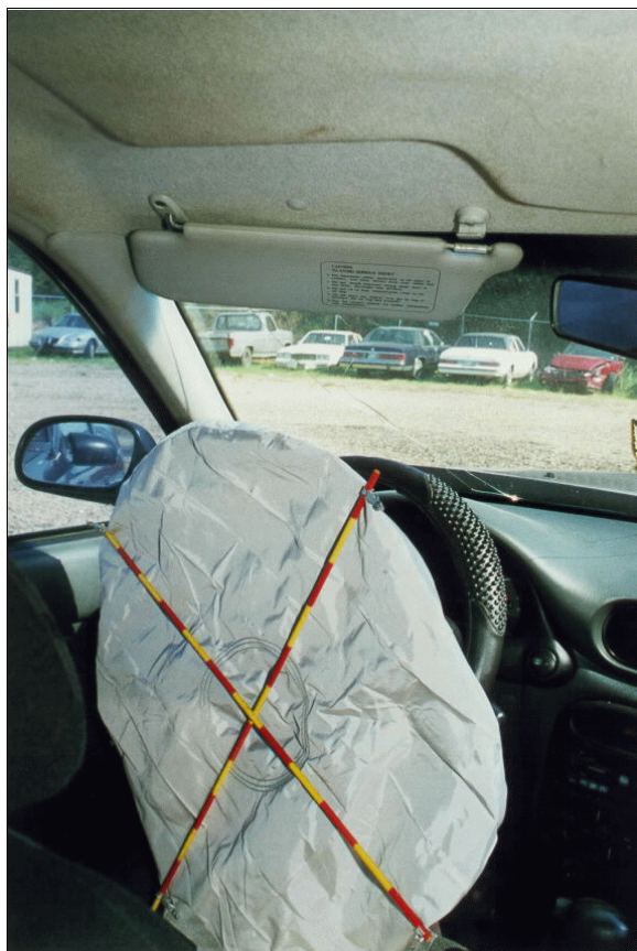
Figure 7: Vertical view of case vehicle's driver seating area showing no apparent visible contact evidence on deployed air bag or to greenhouse areas (case photo #26)
