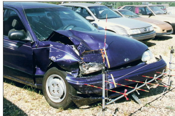
Figure 5: Case vehicle's front right impact showing restricted right front tire and induced damage to right fender and windshield (case photo #17)
