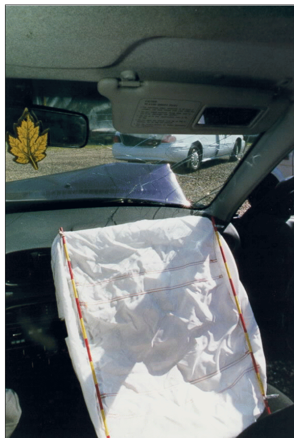
Figure 8: Case vehicle's front right passenger seating area showing no apparent visible contact evidence on deployed air bag's front surface and greenhouse areas, except for stress fractures to right windshield's glazing (case photo #29)
