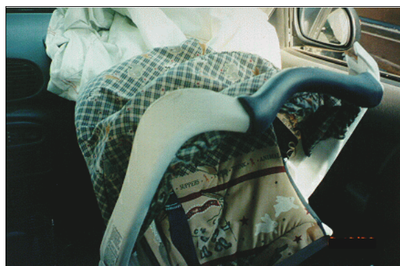
Figure 16: On-scene view of case vehicle's rear facing child safety seat at final rest; Note: carrying handle is in up position and sun umbrella is extended (case photo #55)
