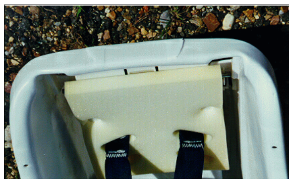
Figure 13: Overhead view of case vehicle's RFCSS showing cracks to top of back support from contact with front right air bag module's cover flap (case photo #43)
