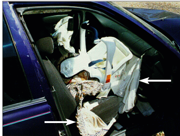
Figure 14: On-scene view of position of case vehicle's front right, rear facing child safety seat (RFCSS) in vehicle; Note: front right air bag module's cover flap contacted back of seat's shell and seat cover and sun umbrella have been pulled away from shell (case photo #54)
