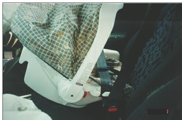
Figure 15: On-scene view of case vehicle's, improperly secured (i.e., by lap belt only), front right rear facing child safety seat (RFCSS); Note: carry handle is in up position (case photo #59)
