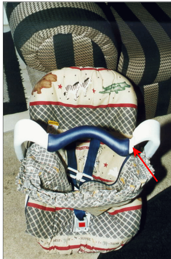
Figure 12: Rear Facing Child Safety Seat (RFCSS) used by case vehicle's front right passenger; Note: broken carry handle (case photo #40)
