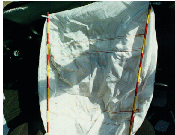
Figure 11: Case vehicle's front right air bag; Note: no apparent physical evidence of contact was found (case photo #36)
