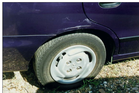
Figure 6: Damage to case vehicle's right quarter panel from sideswiping mailbox (case photo #14)
