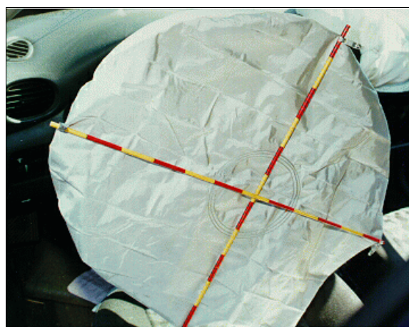
Figure 9: Case vehicle's tethered and vented driver air bag; Note: no apparent physical evidence of contact was found (case photo #25)
