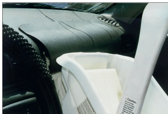
Figure 17: On-scene view showing proximity of case vehicle front right air bag module's cover flap and cracked back edge of RFCSS (case photo #58)
