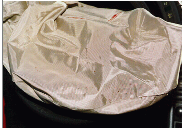
Figure 15: Case vehicle's deployed driver air bag showing hair and blood spray from driver towards bottom of air bag; Note: steering wheel inverted at time of deployment (case photo #26)
