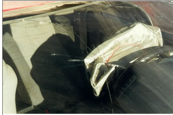
Figure 7: Exterior view of front right passenger's contact to case vehicle's right center windshield (case photo #19)
