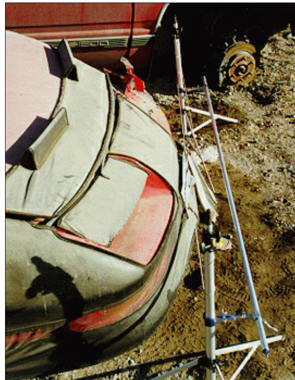
Figure 12: Case vehicle's minimally deformed front viewed along front reference line from right (case photo #20)
