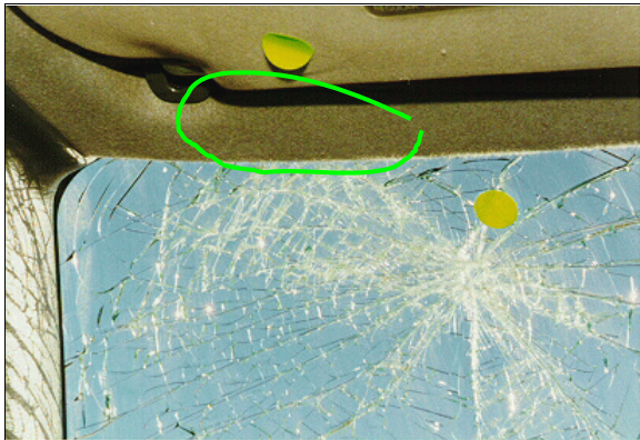
Figure 9: Close-up of case vehicle's front left header area showing driver's head strike to windshield, header, and sun visor; Note: hair hanging down (case photo #30)
