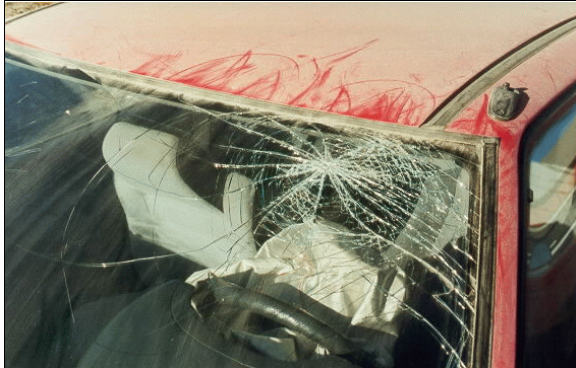
Figure 6: Exterior view of driver's contact to case vehicle's upper left windshield (case photo #14)
