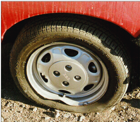
Figure 11: Close-up view of case vehicle's right front wheel showing rim and tire damage from curb impact (case photo #18)
