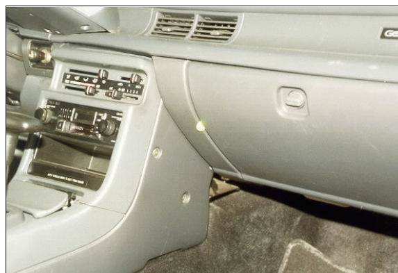
Figure 17: Contact evidence to case vehicle's lower right instrument panel from front right passenger (case photo #34)
