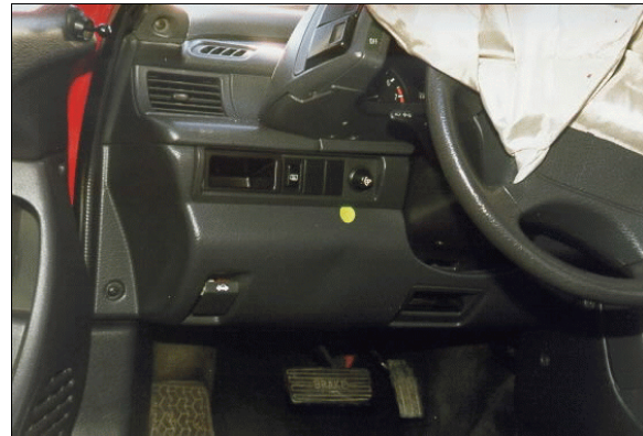
Figure 10: Contact evidence on case vehicle's driver knee bolster, left of steering column (case photo #23)
