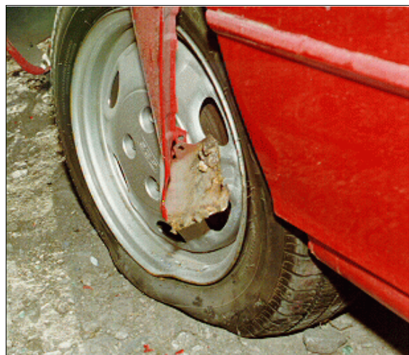
Figure 13: Close-up of case vehicle's left front wheel, viewed from rear of left, showing rim damage from fire hydrant impact (case photo #13)
