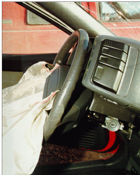
Figure 8: Side view of case vehicle's steering wheel and column pushed forward into instrument panel from driver loading (case photo #29)
