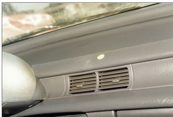
Figure 16: Contact evidence on case vehicle's center instrument panel from front right passenger (case photo #35)
