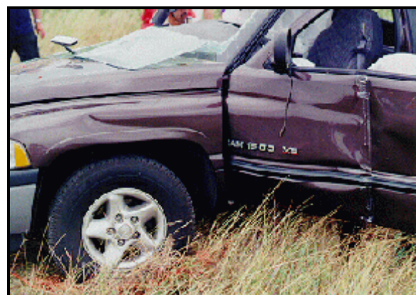
Figure 4: Road sign post impact to Dodge's left front door; Note: damage extended to top of door window frame (case photo #07)
