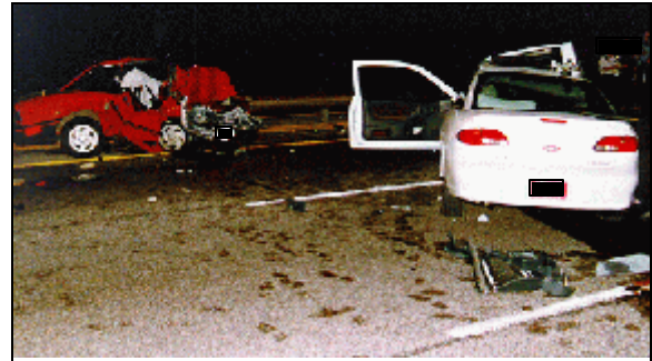
Figure 7: Vehicle #2's induced right side damage; Note: shortened right wheelbase (case photo #19)
