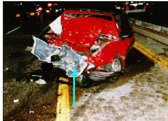
Figure 6: Vehicle #2’s front damage; Note: arrow denotes case vehicle’s front bumper fascia embedded in vehicle #2’s front bumper (case photo #15)
