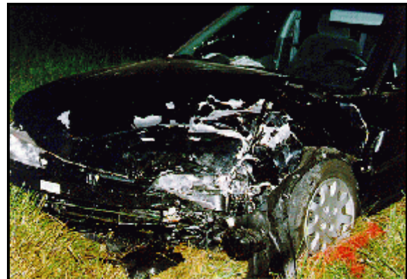
Figure 6: Vehicle #1's front left damage; Note: missing front bumper fascia and deployed dual front air bags (case photo #19)
