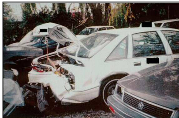
Figure 5: Back and right side of the Caprice, damage caused by the front of the Saturn (case photo #05)
