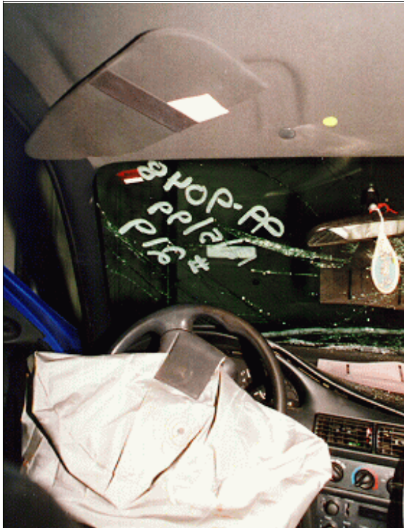
Figure 14: Case vehicle's driver seating area showing deployed driver air bag and cloth transfer on air bag module's left cover flap; Note: steering wheel has been rotated approximately 100 degrees clockwise in this photo (case photo #38)
