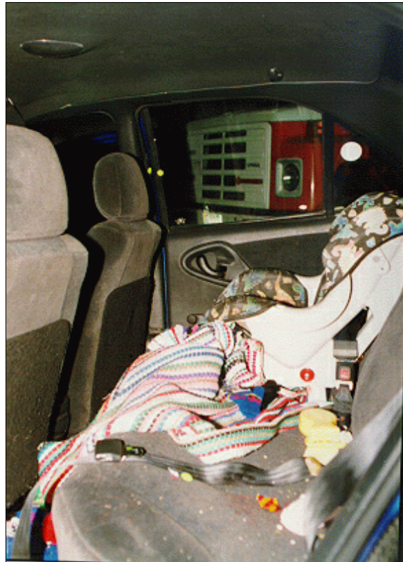
Figure 19: Case vehicle's back left seating area and contacted "B"-pillar (i.e., yellow dots); Note: unused, secured, child safety seat in back right position (case photo #58)
