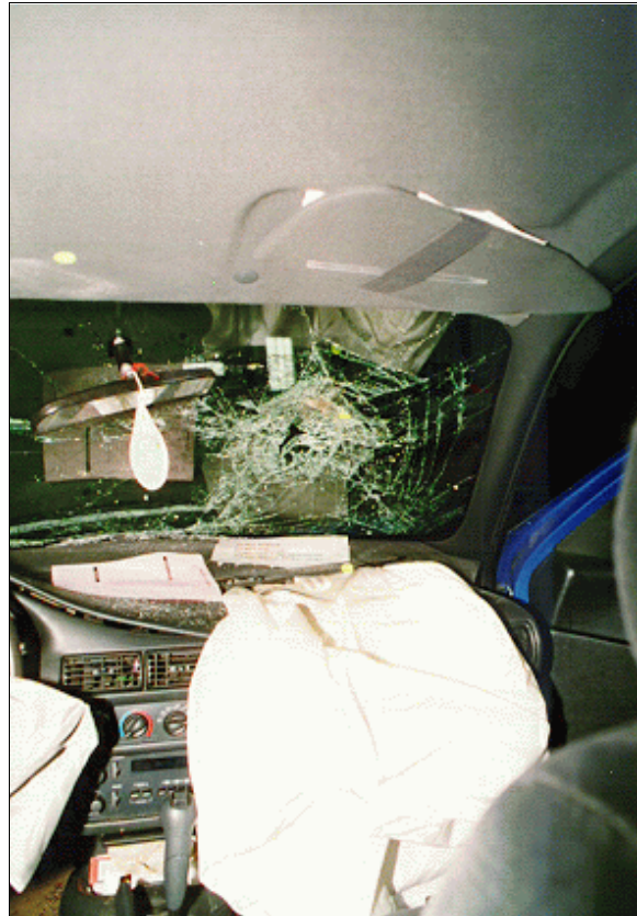
Figure 12: Case vehicle’s front right passenger seating area showing occupant contacts to roof, windshield, top of air bag and air bag module’s cover flap (case photo #48)
