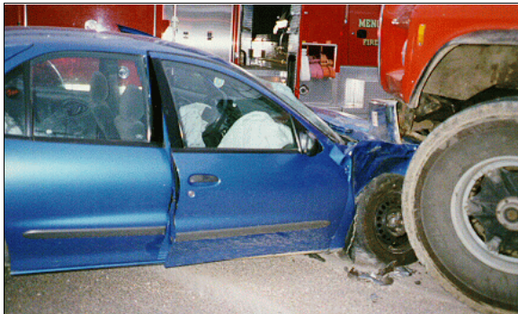
Figure 8: On-scene close-up of case vehicle under Ford's front bumper; Note: deployed driver and front right passenger air bags (case photo #15)
