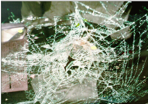
Figure 13: Close-up of interior surface of case vehicle’s holed right windshield; Note: windshield contacted by head of front unseated passenger (case photo #50)
