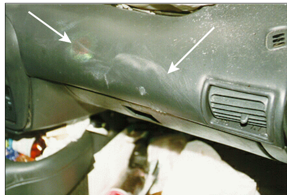
Figure 11: Apparent occupant cloth transfers to case vehicle's right instrument panel from front unseated passenger (case photo #47)
