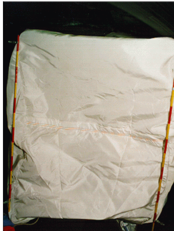
Figure 18: Case vehicle's front right passenger air bag showing no apparent evidence of contact from front unseated passenger (case photo #57)
