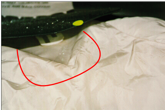
Figure 17: Close-up of case vehicle front right air bag module's contacted cover flap (yellow dot) and faint red and green cloth transfer to top of air bag (case photo #53)
