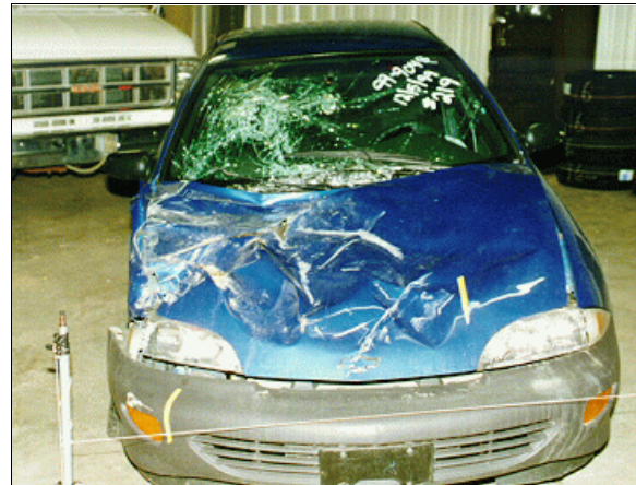
Figure 9: Case vehicle's underride type damage to front and right side from impact with Ford; Note: yellow tape highlights width of hood that was overridden (case photo #17)
