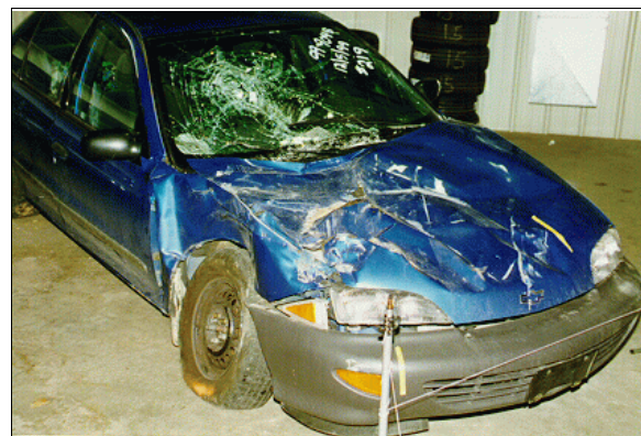
Figure 10: Case vehicle's frontal damage; Note: override type deformation, damaged right front wheel, and starred windshield (case photo #33)
