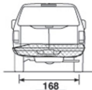
Max. crush to rear at right bumper corner
