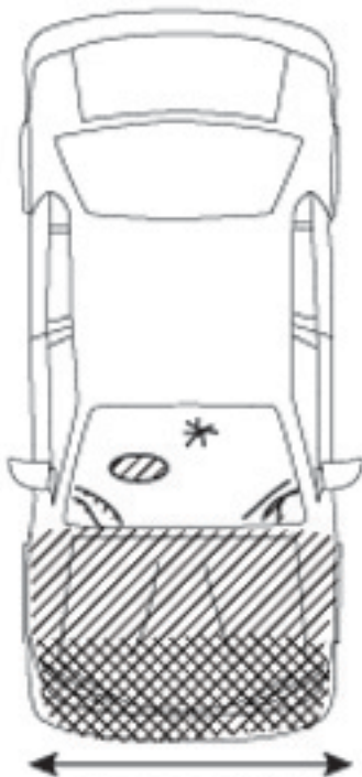
impact #1 144-cm direct damage 31-cm max crush
