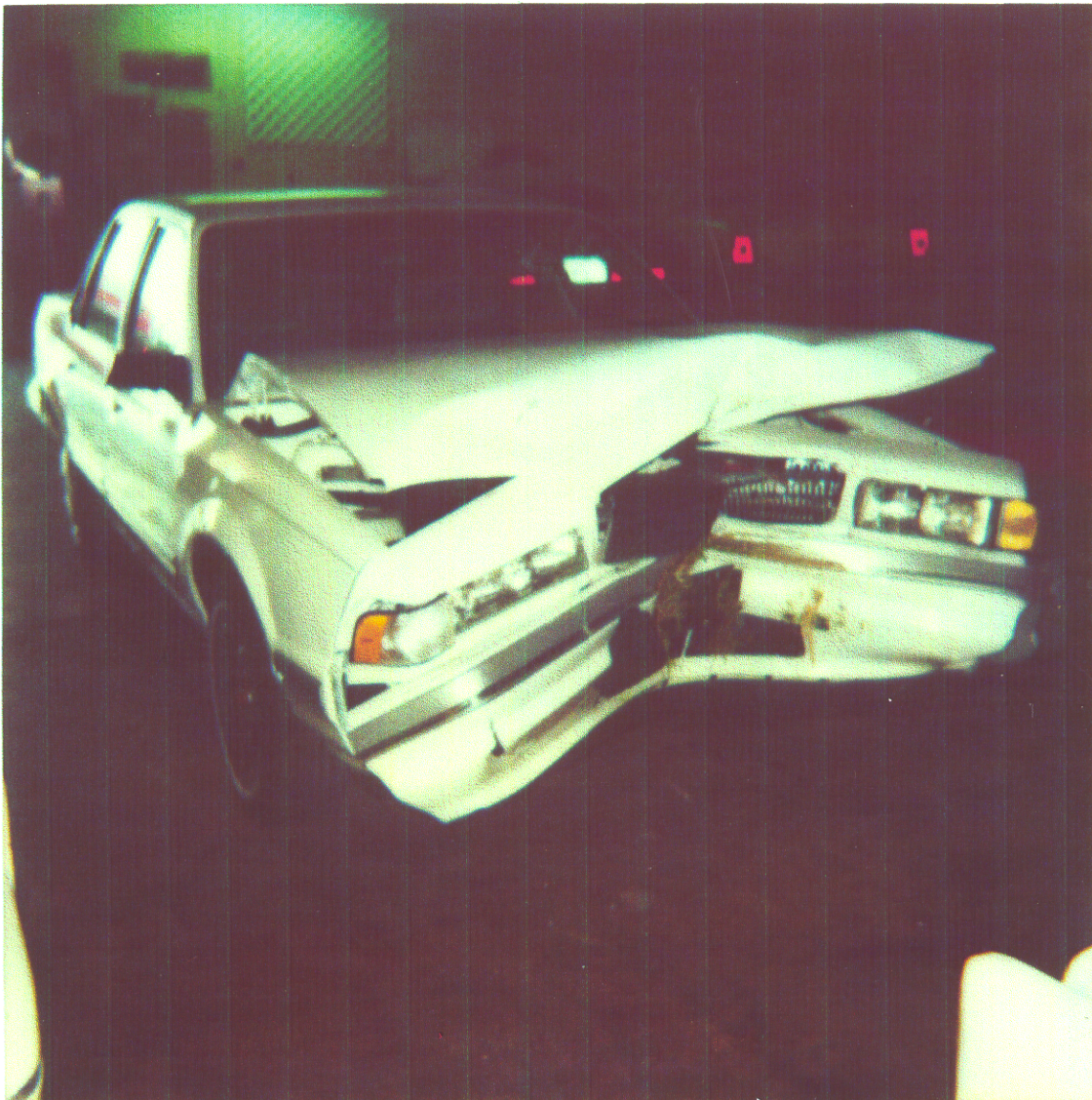
2. Right front three-quarter view showing the extent of frontal crush.
