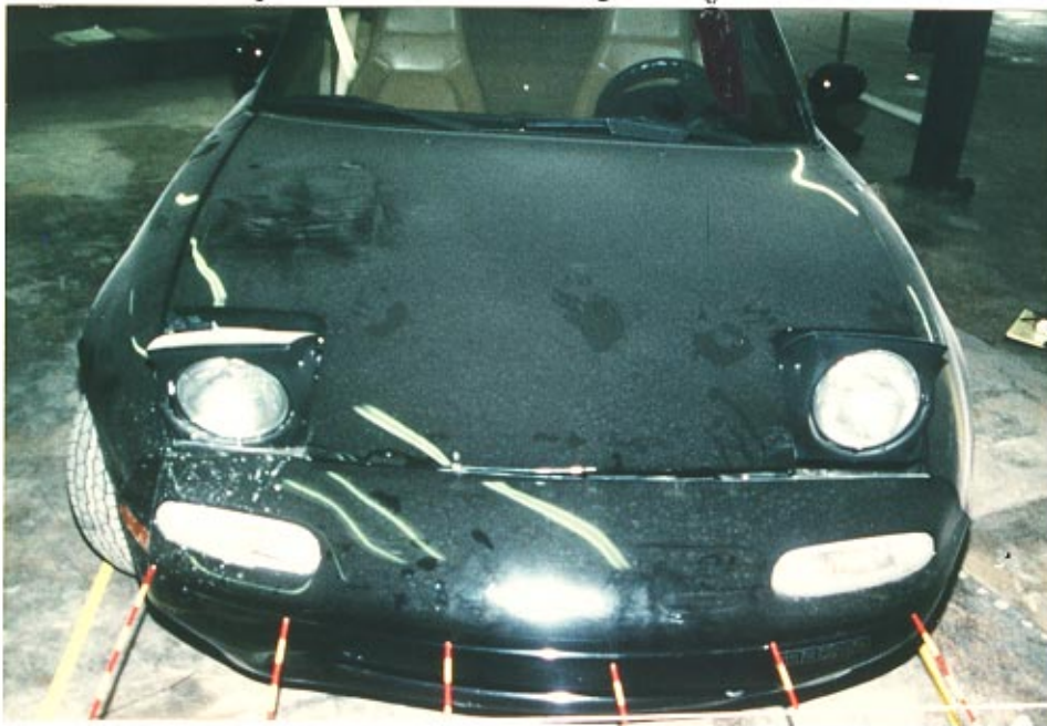
22. Secondary impact damage to the right frontal area.
