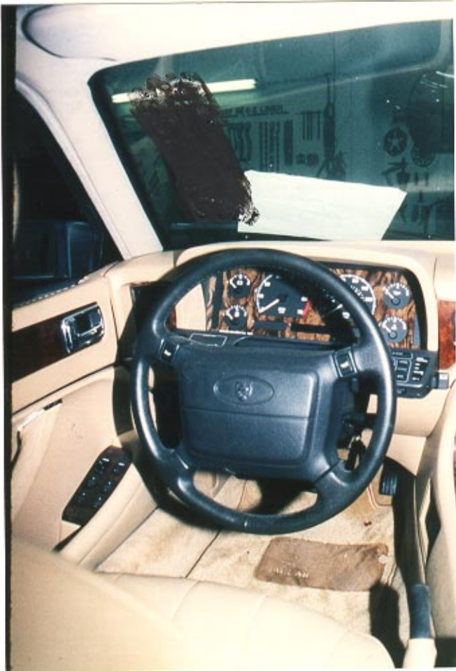
11. Nondeployed driver's side air bag.
