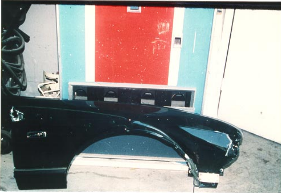
7. Removed and damaged right front fender.
