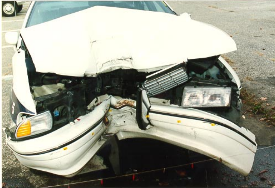
5. Frontal view of the tree impact damage to the Chevrolet Caprice.
