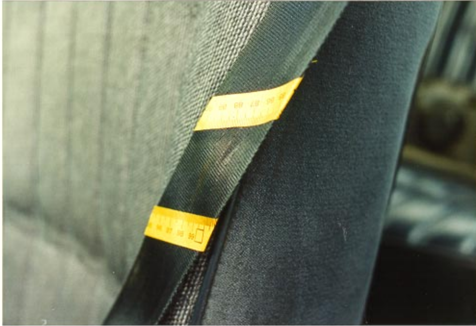
25. D-ring loading transfer on the shoulder belt webbing.
