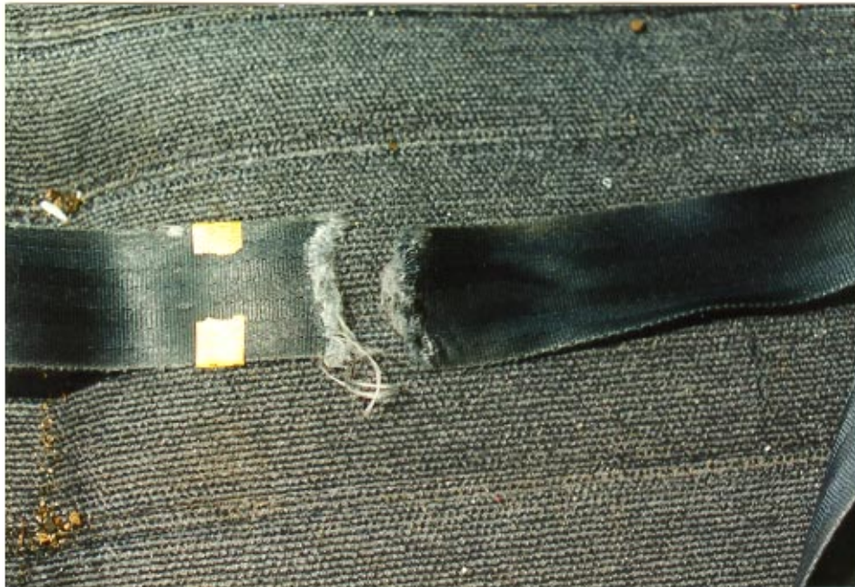
29. & 30. Separation of the belt webbing at the cinch bar location.
