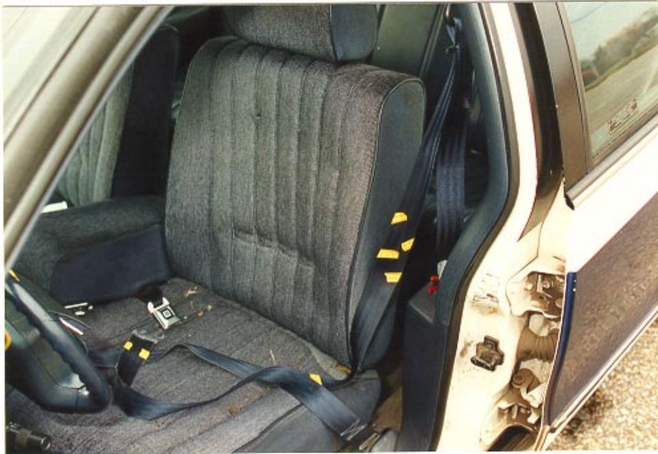
22. Overall view of the manual 3-point lap and shoulder belt system.
