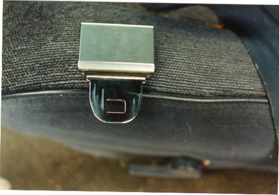
33. Routine usage wear marks on the male tab of the latchplate.
