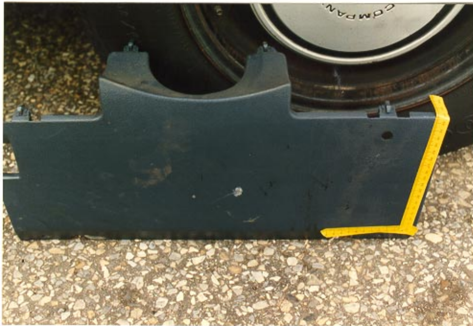
20. Right knee contact (scuff) to the removed knee bolster outer panel.
