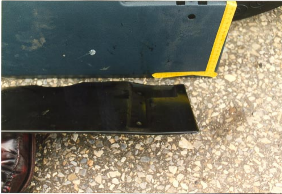
21. Deformation (0.25 cm) from right knee contact to the bolster backer panel.
