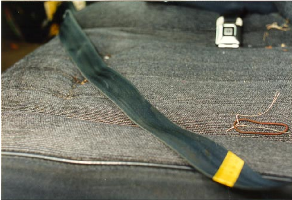
27. Additional view of the loading transfers on the shoulder belt webbing.
