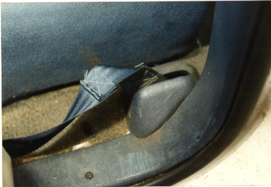
28. Energy management loop and the lower anchorage point of the driver's side belt webbing.
