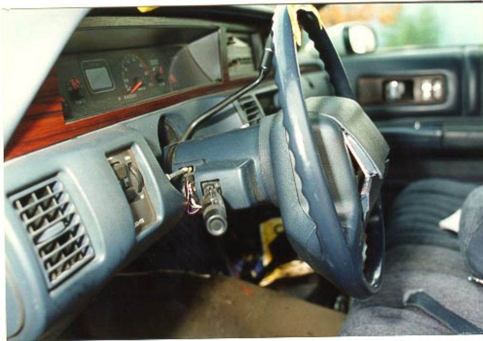
17. Compression of the energy absorbing steering column.
