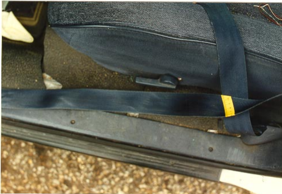
26. Driver loading fabric transfers on the shoulder belt webbing.
