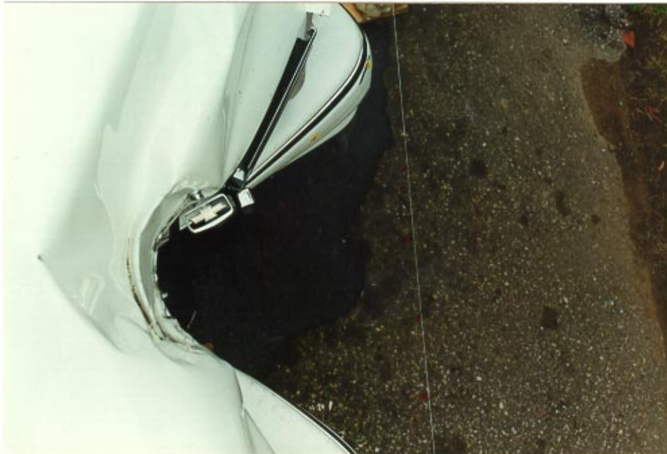
6. Overhead view showing the extent of frontal crush.
