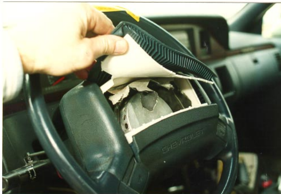
16. Air bag module cover flaps and gas generator with air bag cut from module assembly.
