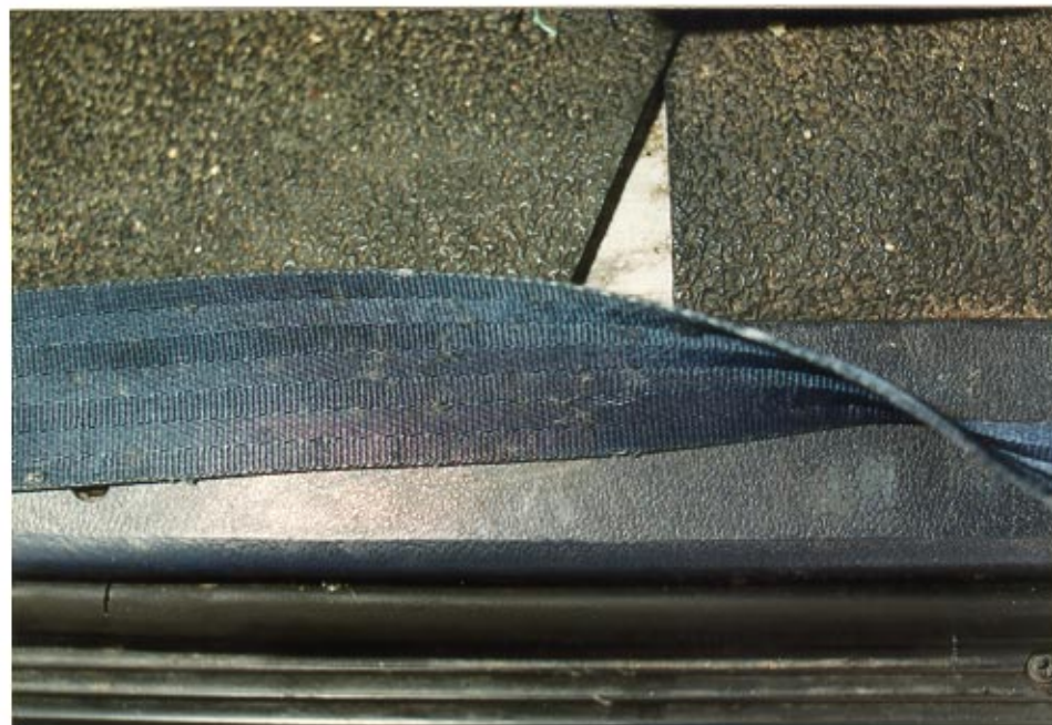
23. & 24. Gouges and scrapes in lap belt webbing from belt becoming caught in door latch/striker.
