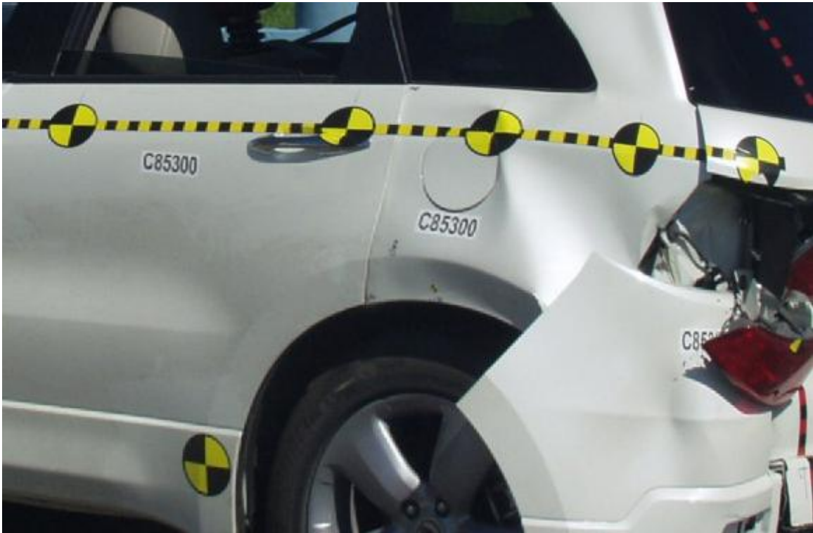
Figure A-36: Post-Test Fuel Filler Cap View
