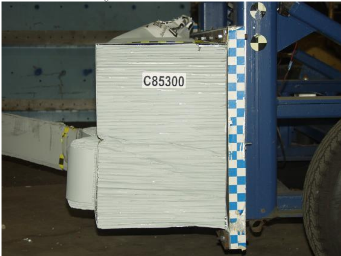
Figure A-22: Post-Test MDB Left Side View
