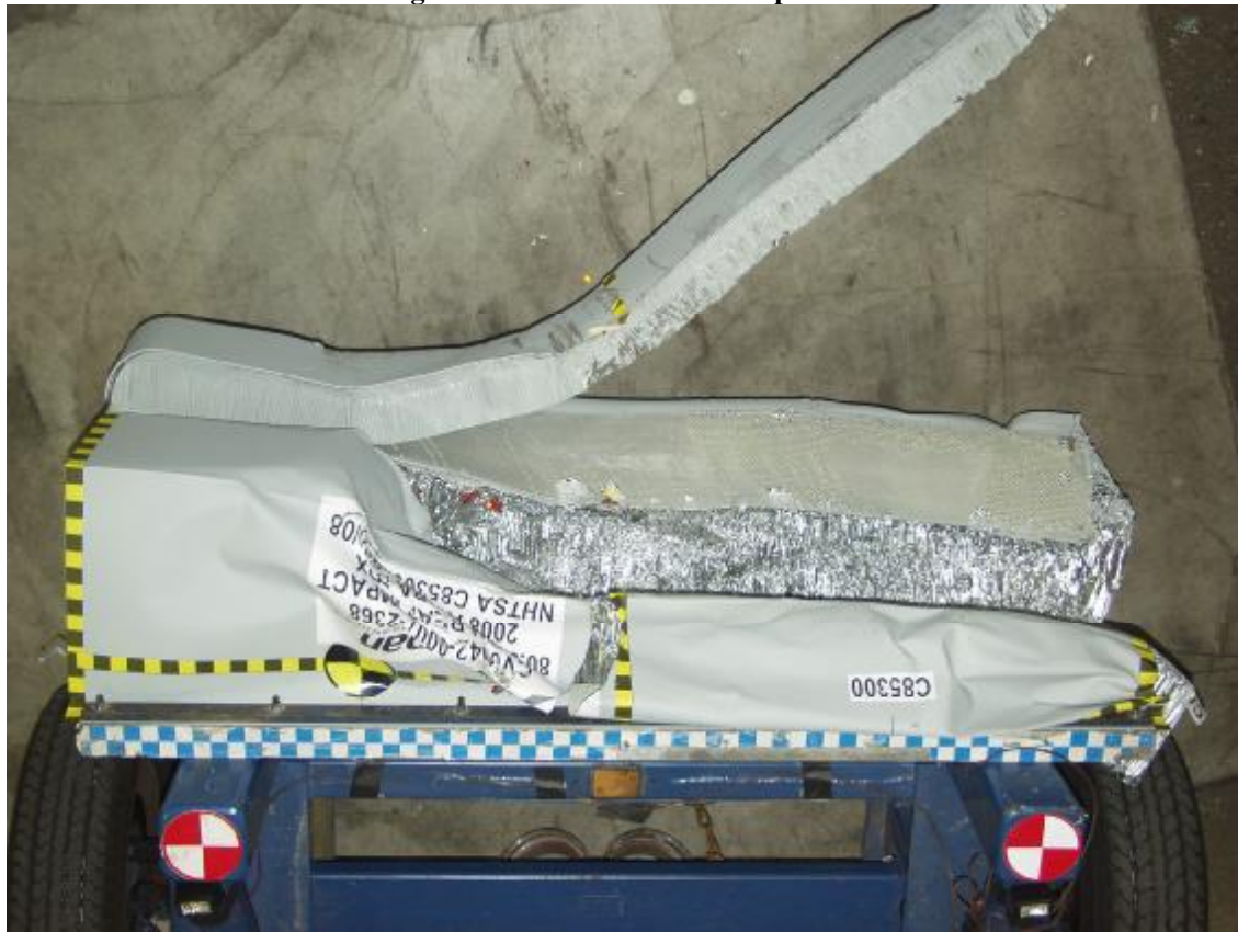
Figure A-26: Post-Test MDB Top View
