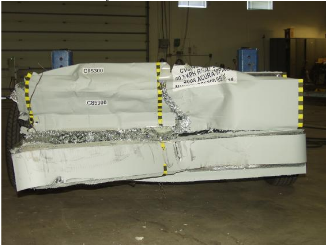
Figure A-20: Post-Test MDB Front View
