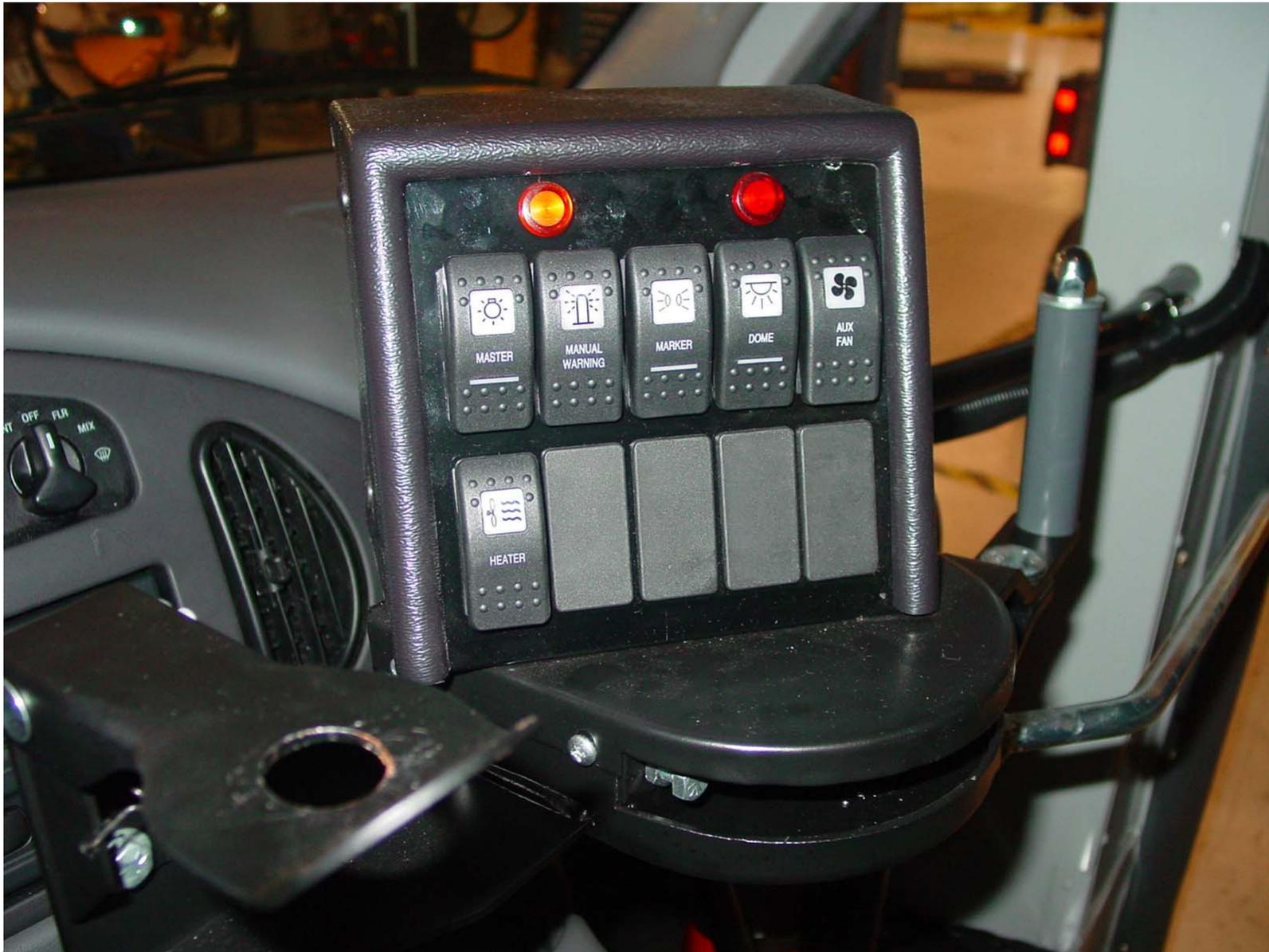
Close Up View of the Switches That Allow Extension of the Stop Signal Arm(s)
