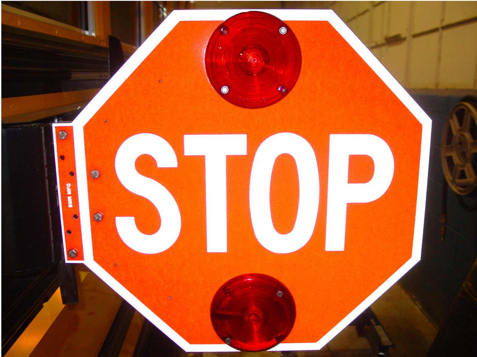
Front Closeup View of Stop Signal Arm
