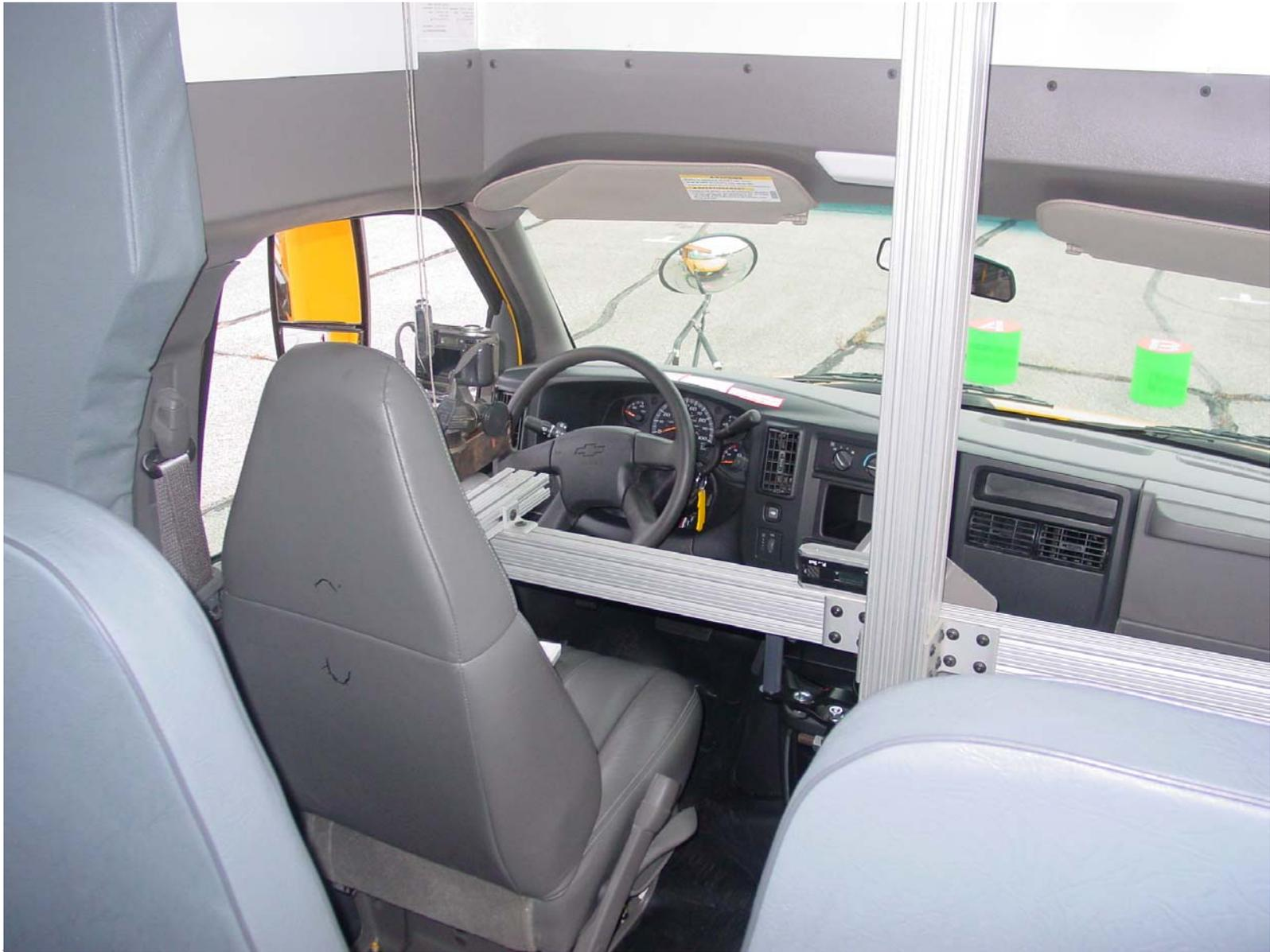
Field of View Instrument Setup
