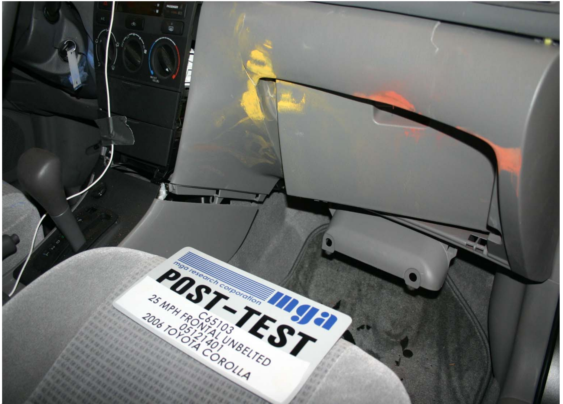
Post-Test Passenger Dummy Knee Contact
