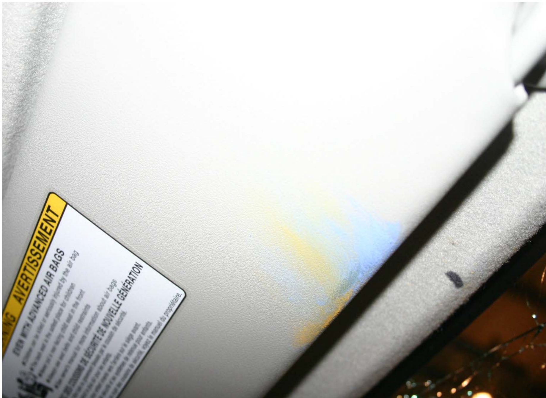
Post-Test Passenger Dummy Head Contact View (visor)
