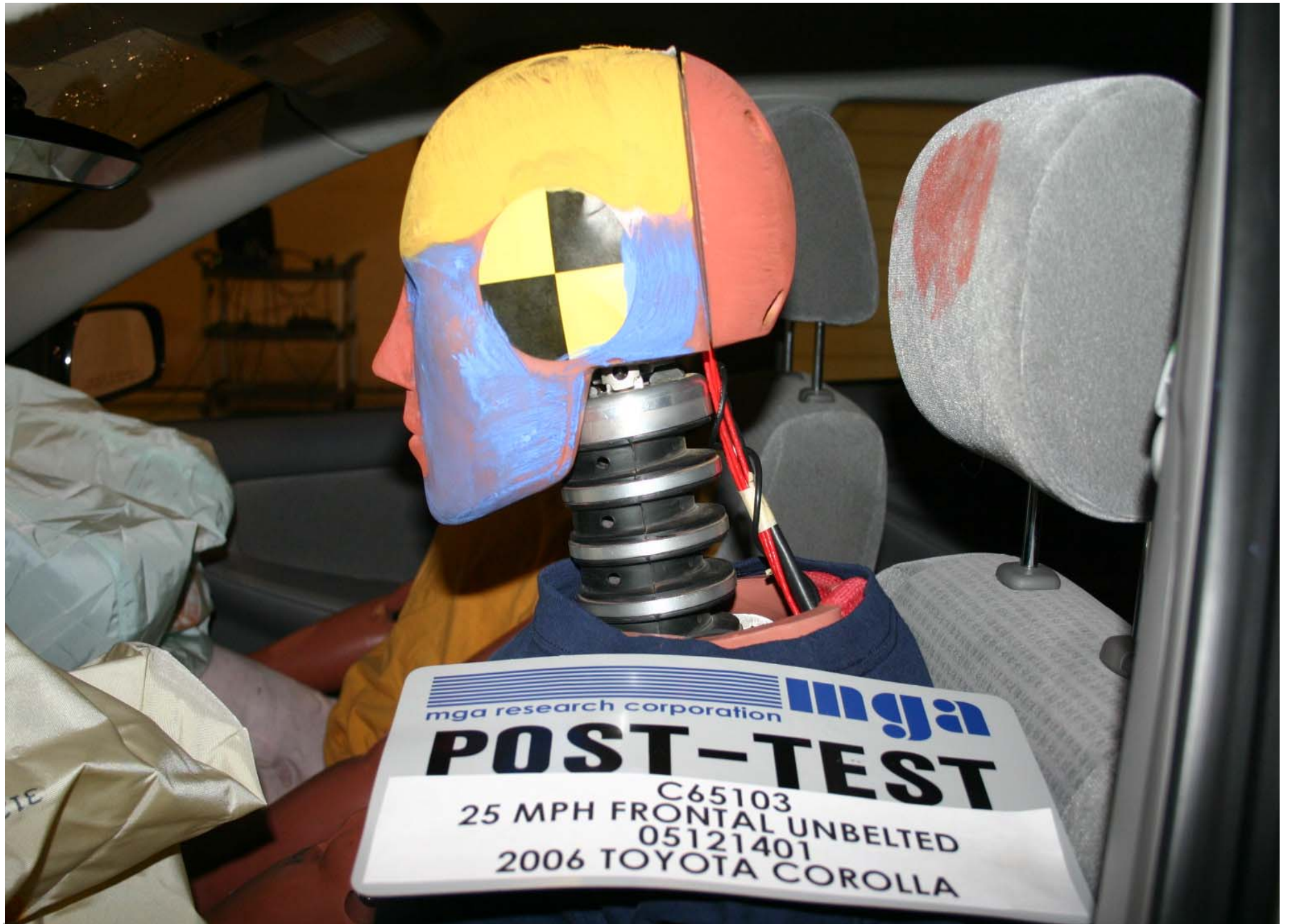
Post-Test Driver Dummy Head Contact (headrest)
