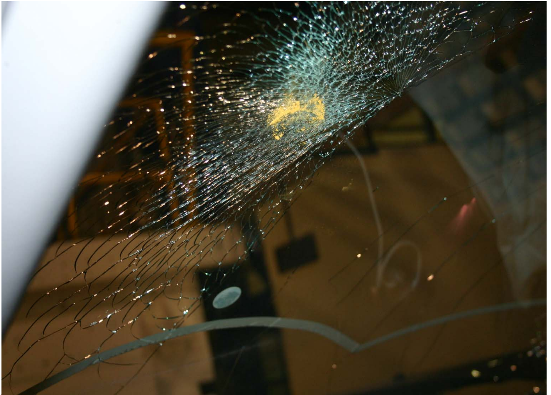
Post-Test Driver Dummy Head Contact (windshield)
