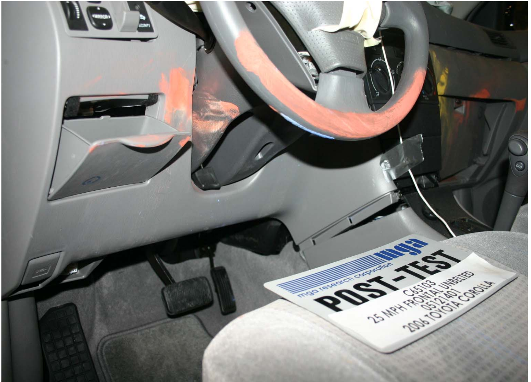
Post-Test Driver Dummy Knee Contact
