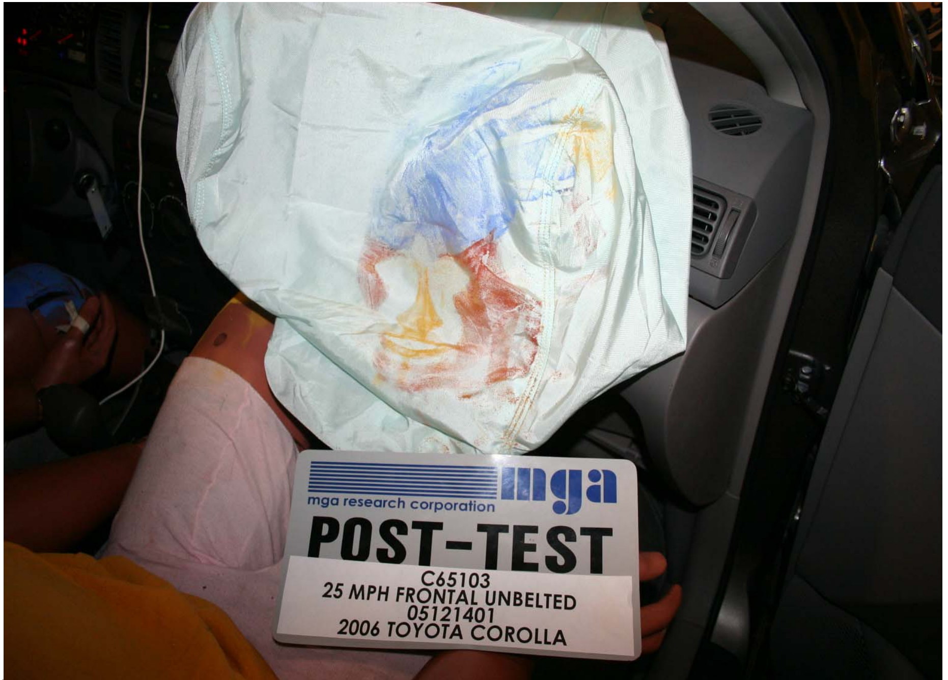
Post-Test Passenger Dummy Airbag Contact
