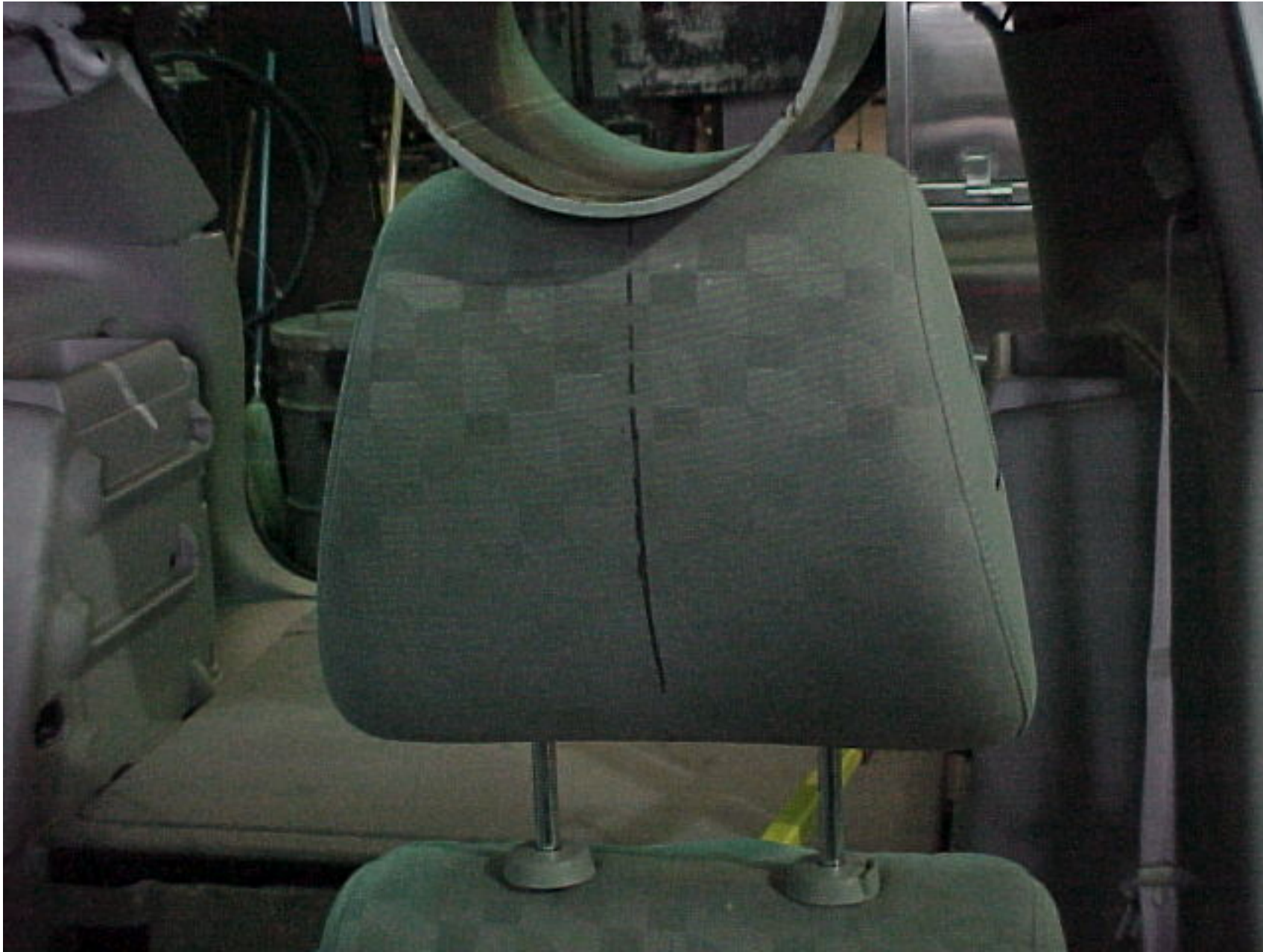
FIGURE 5.12 10% POST LOAD, HEIGHT RETENTION, DRIVER #1
