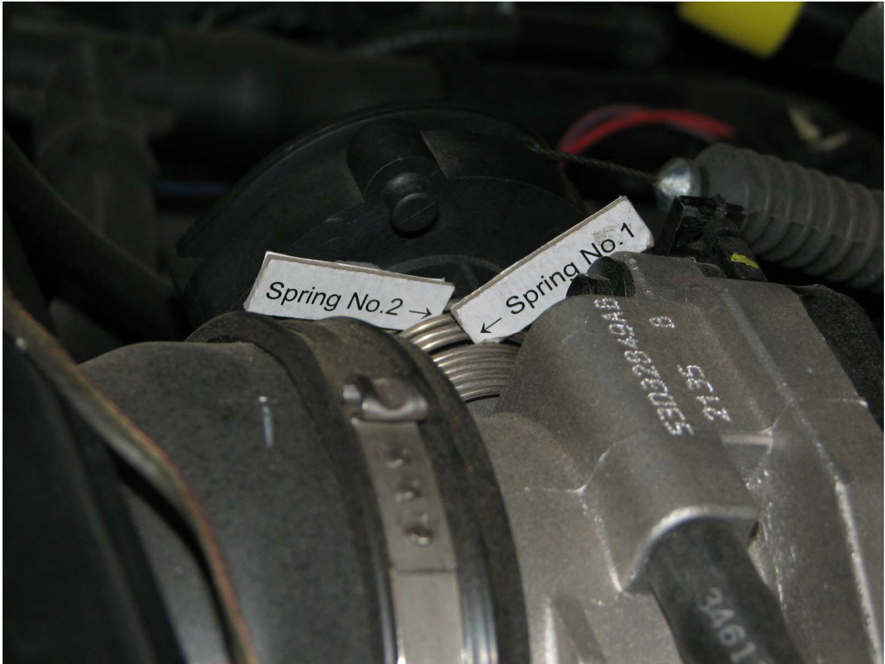
2006 DODGE DAKOTA Figure A-8: Spring 1 and 2 Located on Vehicle's Accelerator Control System (Throttle Body) NHTSA NO. C60302 FMVSS NO. 124
