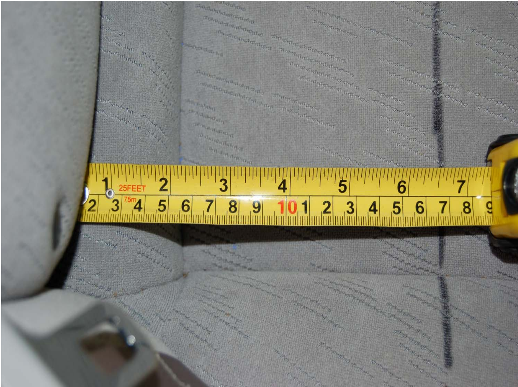
FIGURE 5.28 ROW 2, RIGHT SIDE OUTBOARD SRP MEASUREMENT
