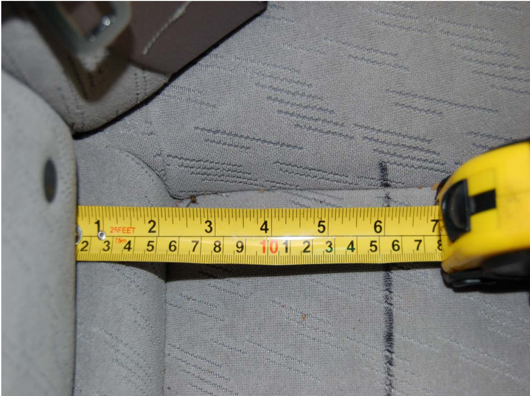
FIGURE 5.26 ROW 2, LEFT SIDE OUTBOARD SRP MEASUREMENT
