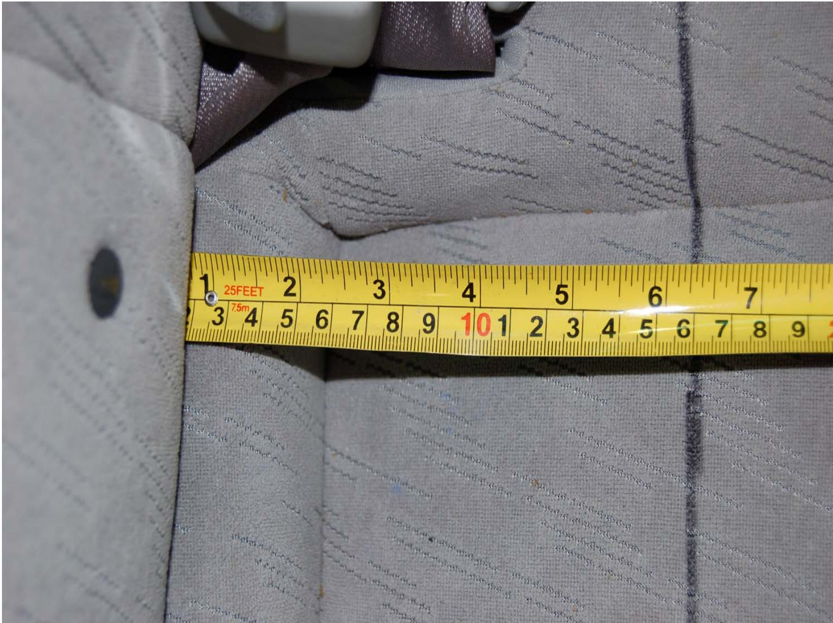
FIGURE 5.29 ROW 2, RIGHT SIDE INBOARD SRP MEASUREMENT
