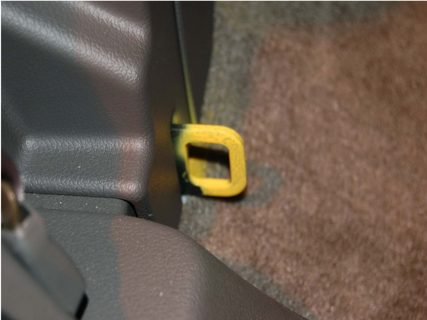
FIGURE 5.14 ROW 2, RIGHT SIDE, TOP TETHER ANCHOR, PRE-TEST
