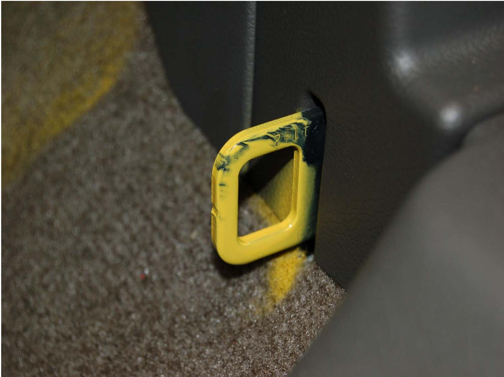
FIGURE 5.9 ROW 2, LEFT SIDE, TOP TETHER ANCHOR, PRE-TEST
