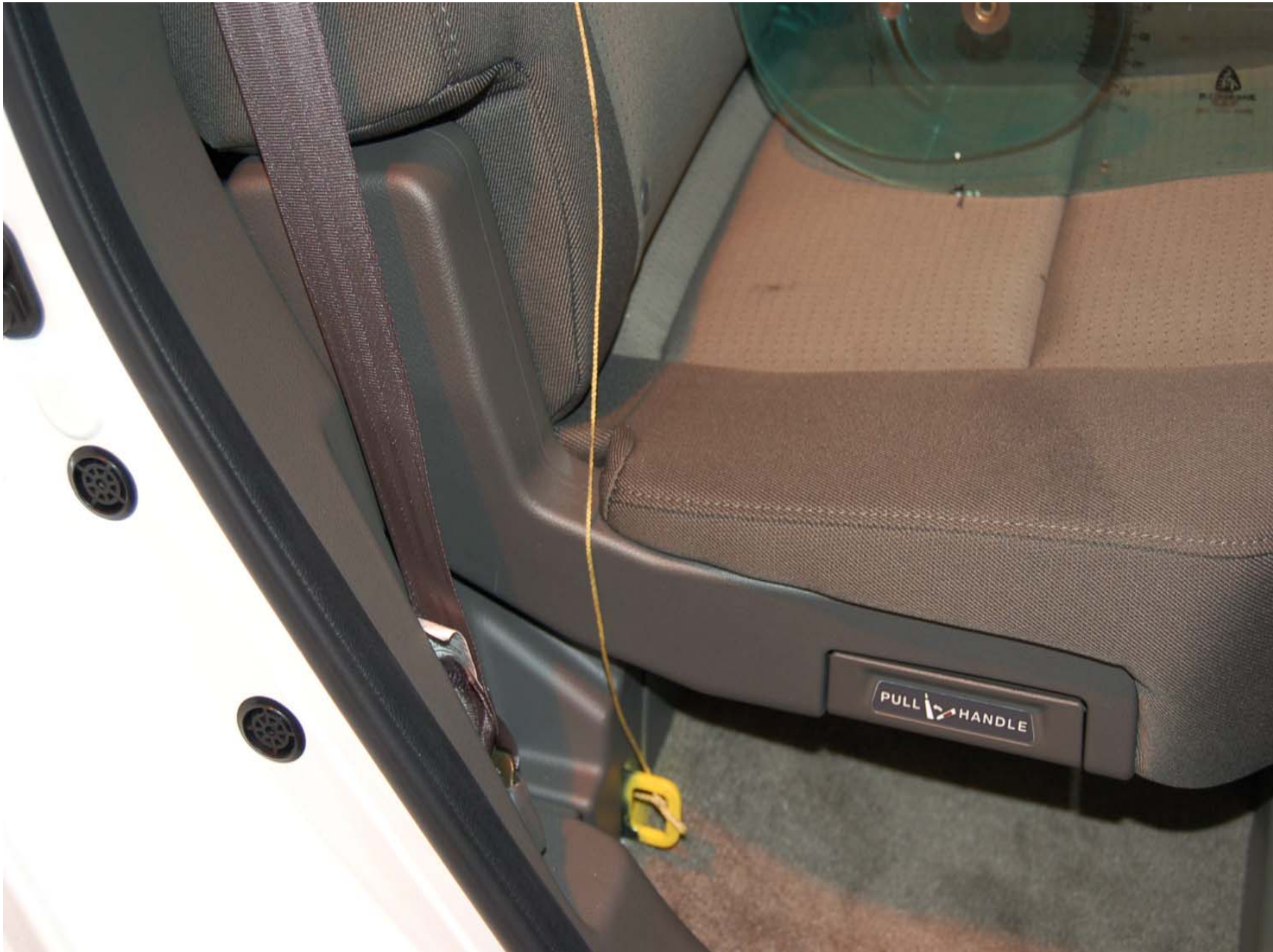
FIGURE 5.23 ROW 2, RIGHT SIDE TETHER ROUTING
