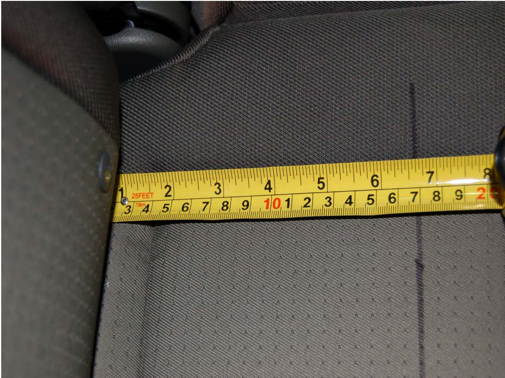
FIGURE 5.41 ROW 2, RIGHT SIDE INBOARD SRP MEASUREMENT
