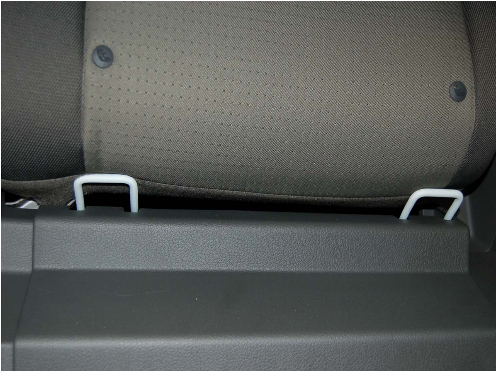
FIGURE 5.12 ROW 2, RIGHT SIDE, LOWER ANCHORS, PRE-TEST
