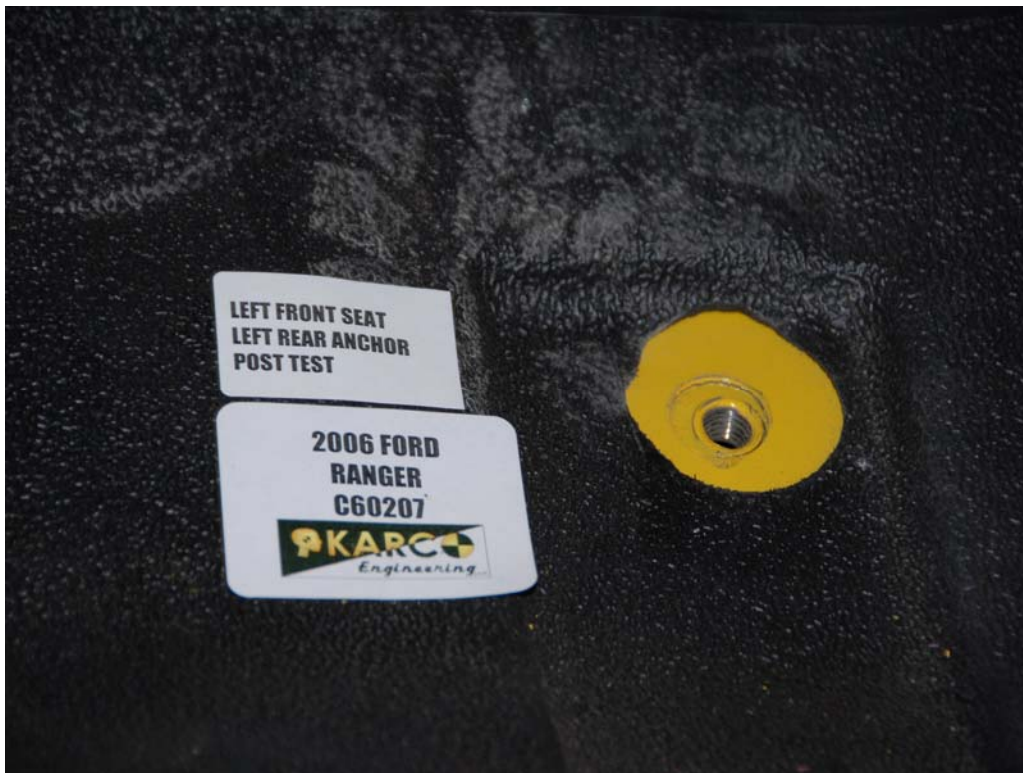
FIGURE 40. Floor Pan Anchor, P1, Post-Test
