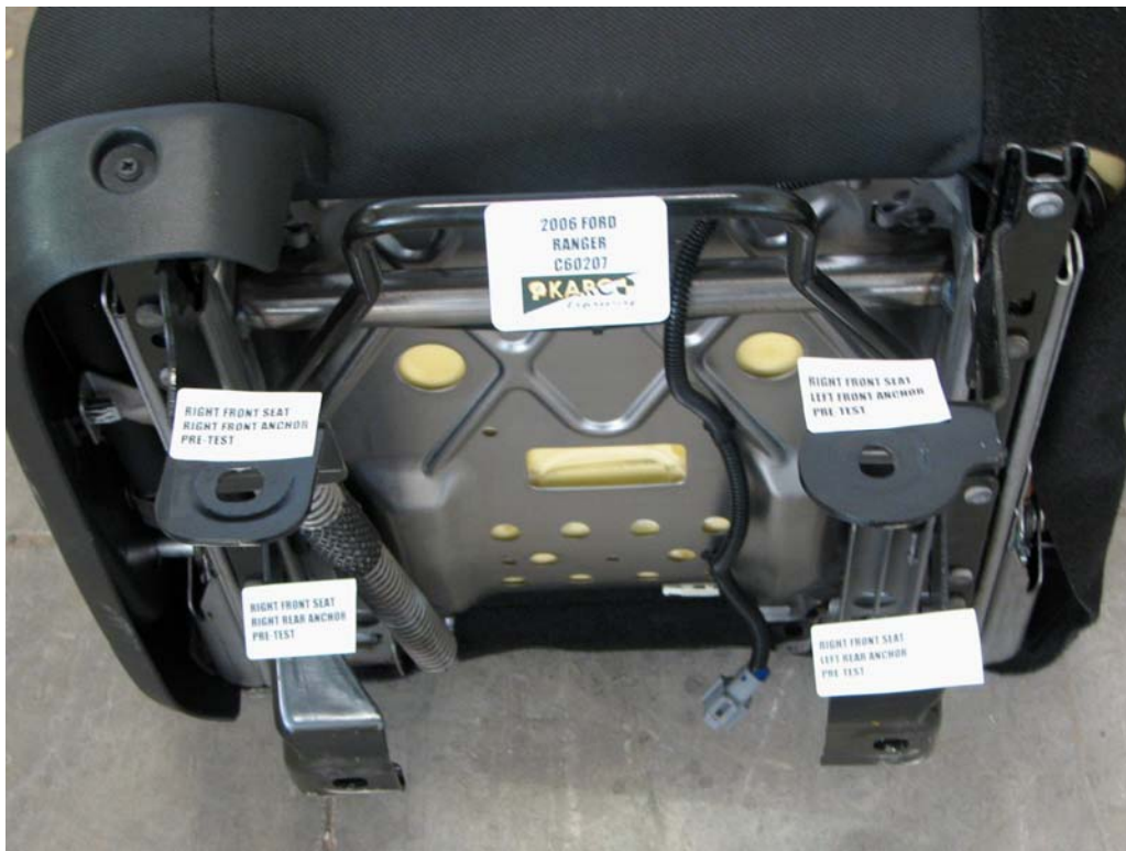
FIGURE 57. Seat Anchors, P2 Overall, Pre-Test
