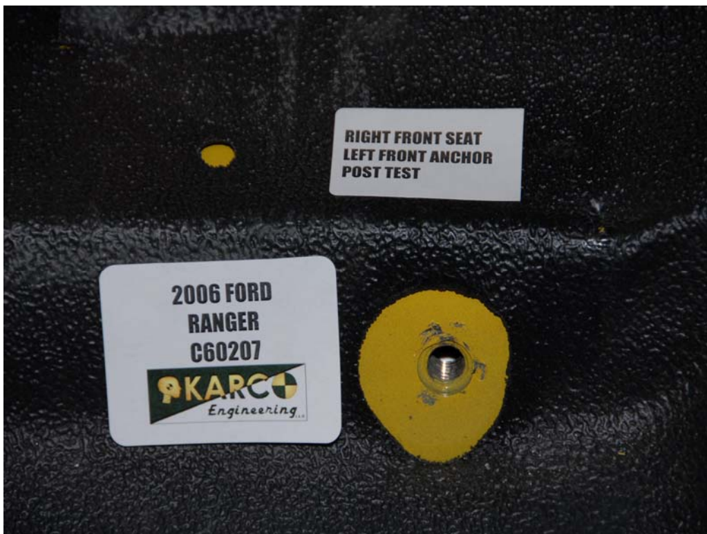
FIGURE 60. Floor Pan Anchor, P2, Post-Test
