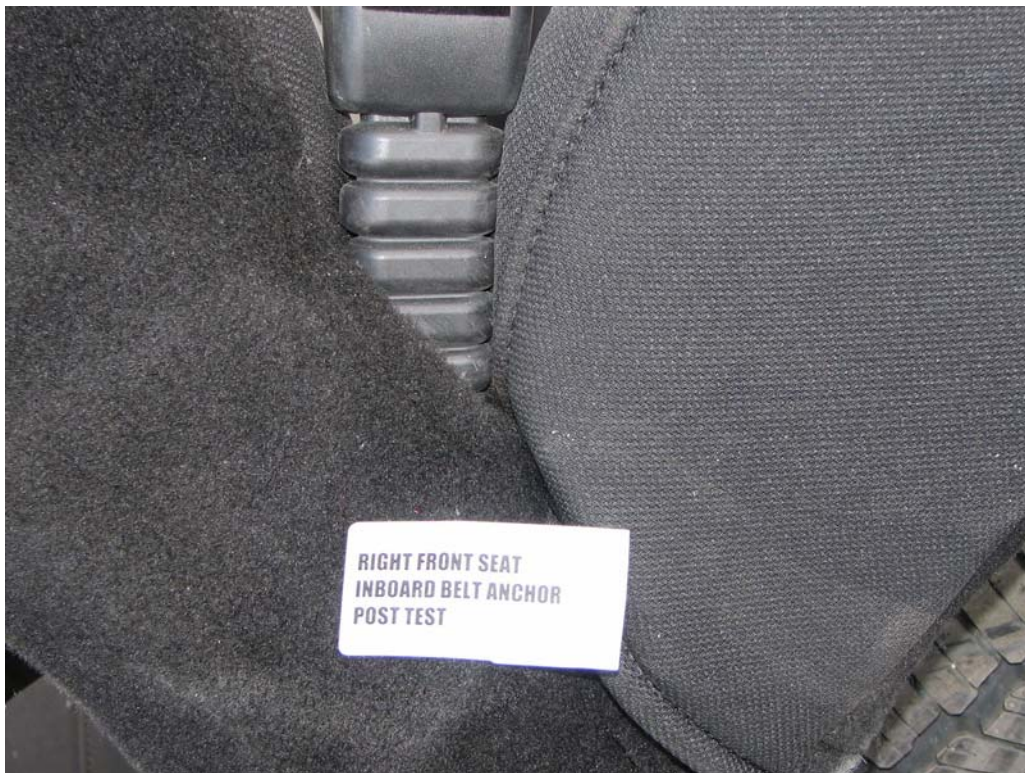
FIGURE 82. Belt Anchor, P2, Post-Test
