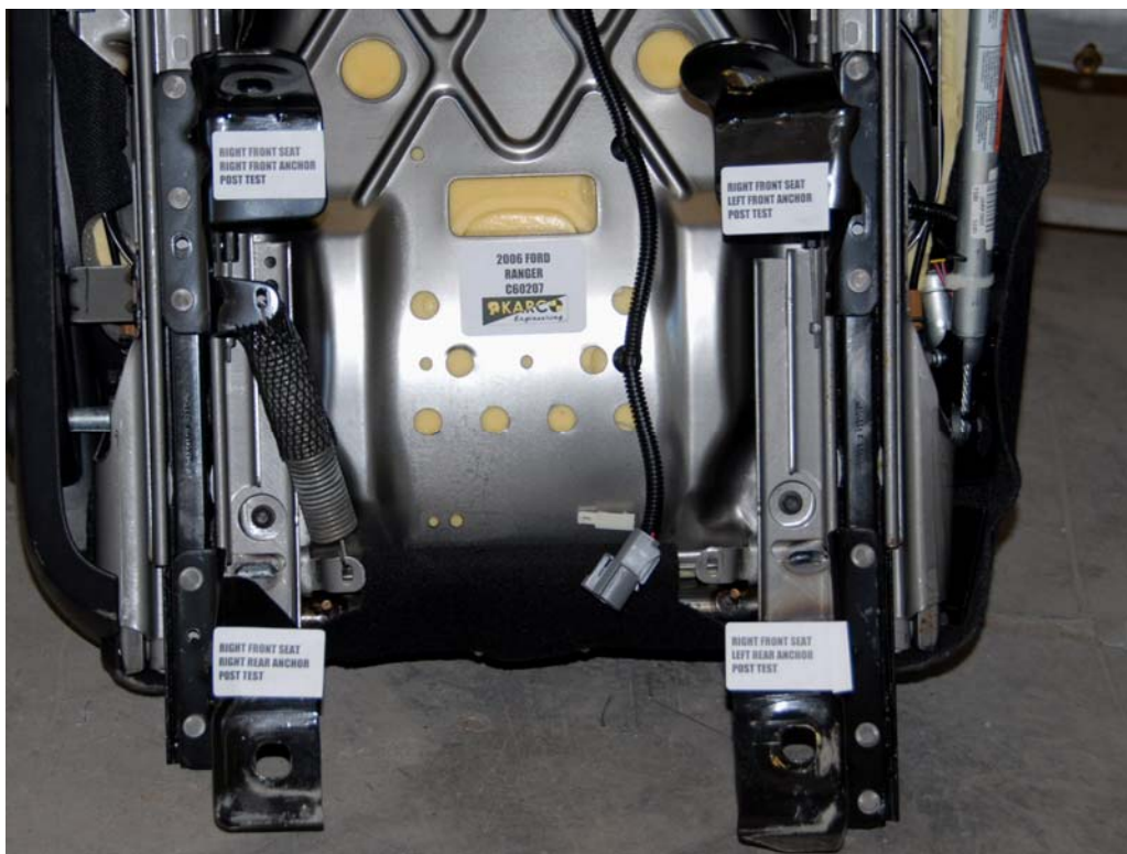
FIGURE 58. Seat Anchors, P2 Overall, Post-Test
