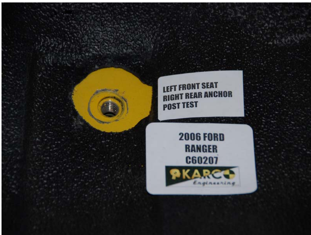
FIGURE 44. Floor Pan Anchor, P1, Post-Test
