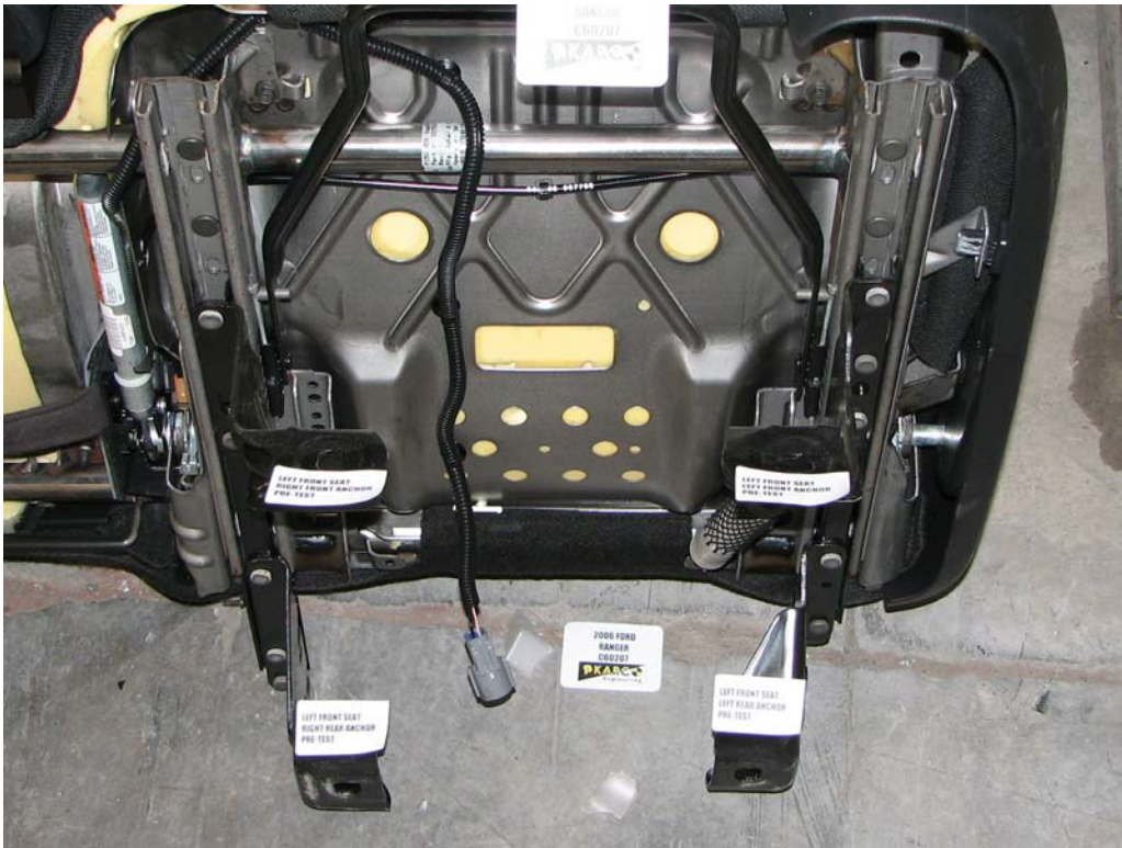
FIGURE 29. Seat Anchors, P1 Overall, Pre-Test
