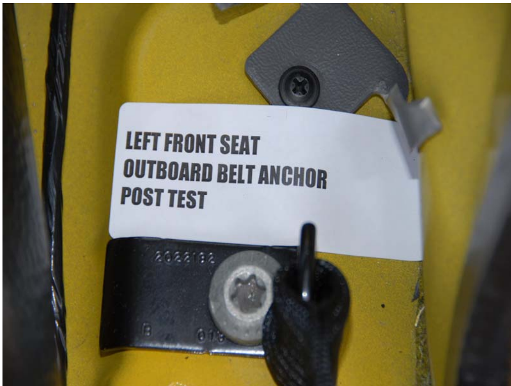
FIGURE 52. Belt Anchor, P1, Post-Test
