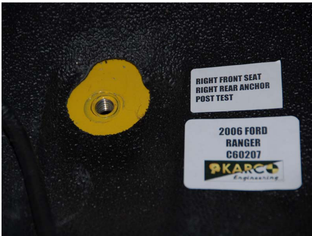
FIGURE 72. Floor Pan Anchor, P2, Post-Test
