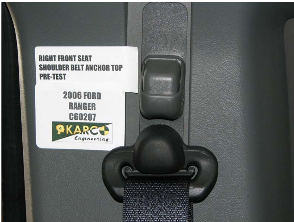
FIGURE 75. Shoulder Belt Anchor, P2, Pre-Test
