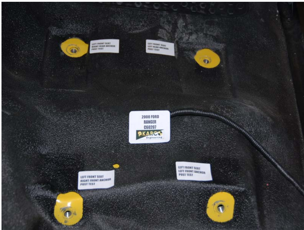
FIGURE 28. Floor Pan Anchors, P1 Overall, Post-Test
