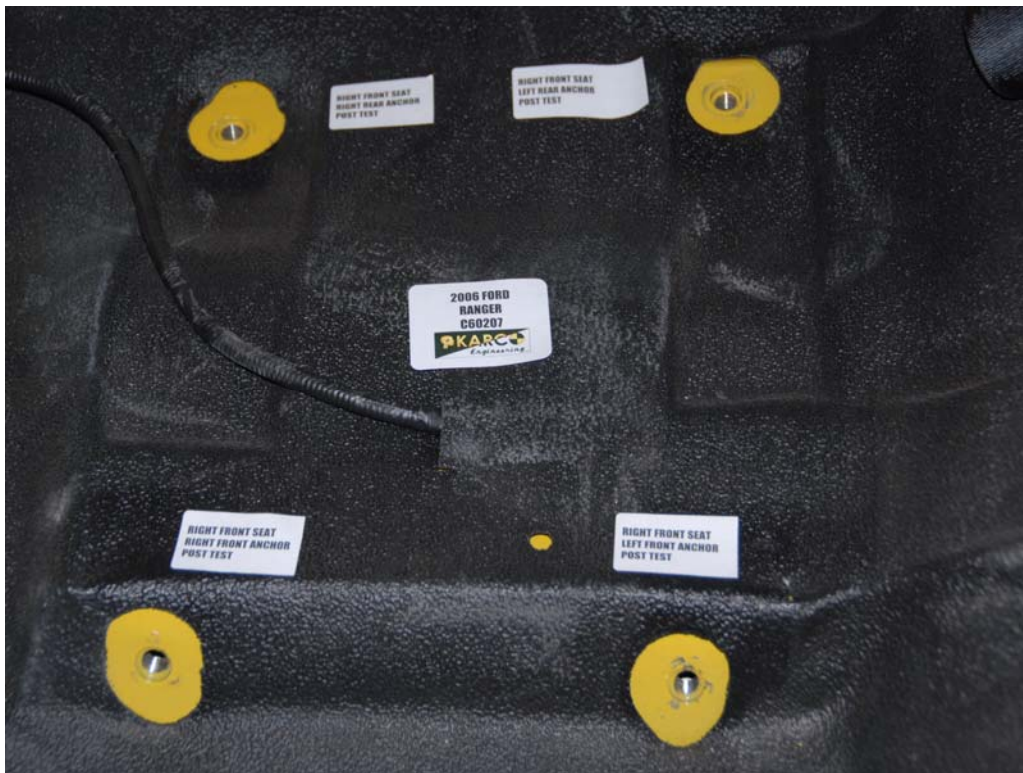
FIGURE 56. Floor Pan Anchors, P2 Overall, Post-Test
