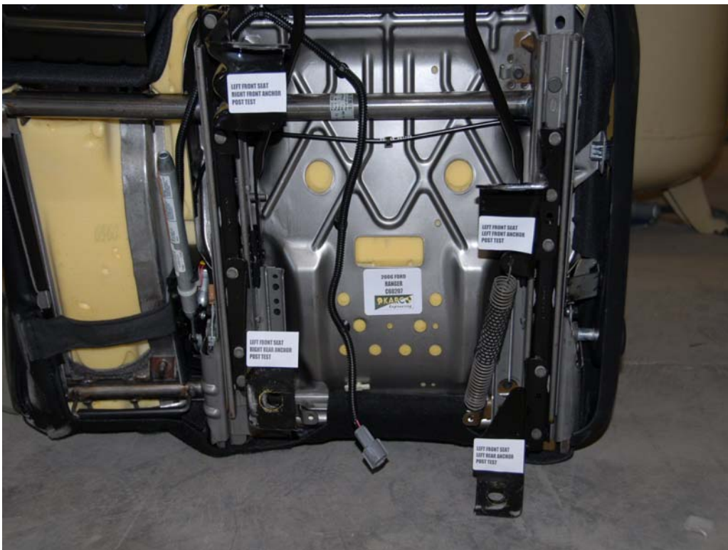
FIGURE 30. Seat Anchors, P1 Overall, Post-Test
