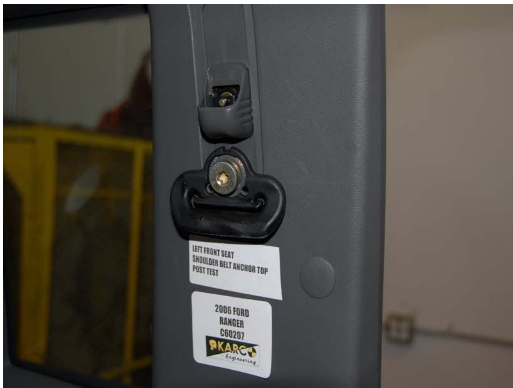
FIGURE 48. Shoulder Belt Anchor, P1, Post-Test
