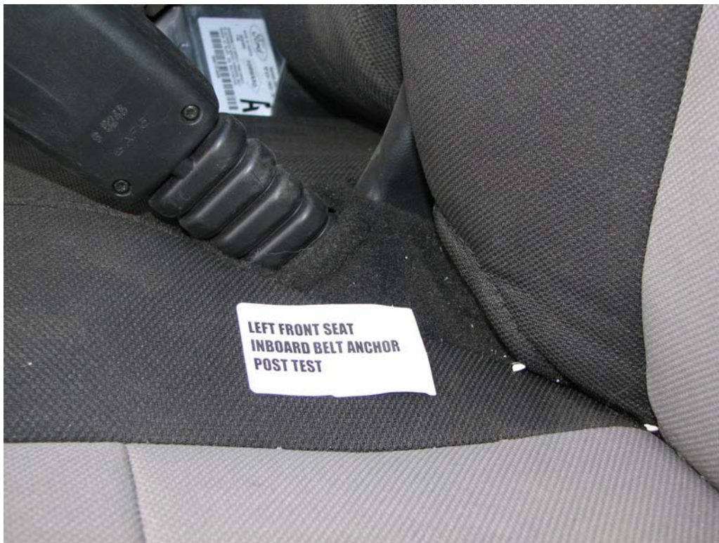
FIGURE 54. Belt Anchor, P1, Post-Test
