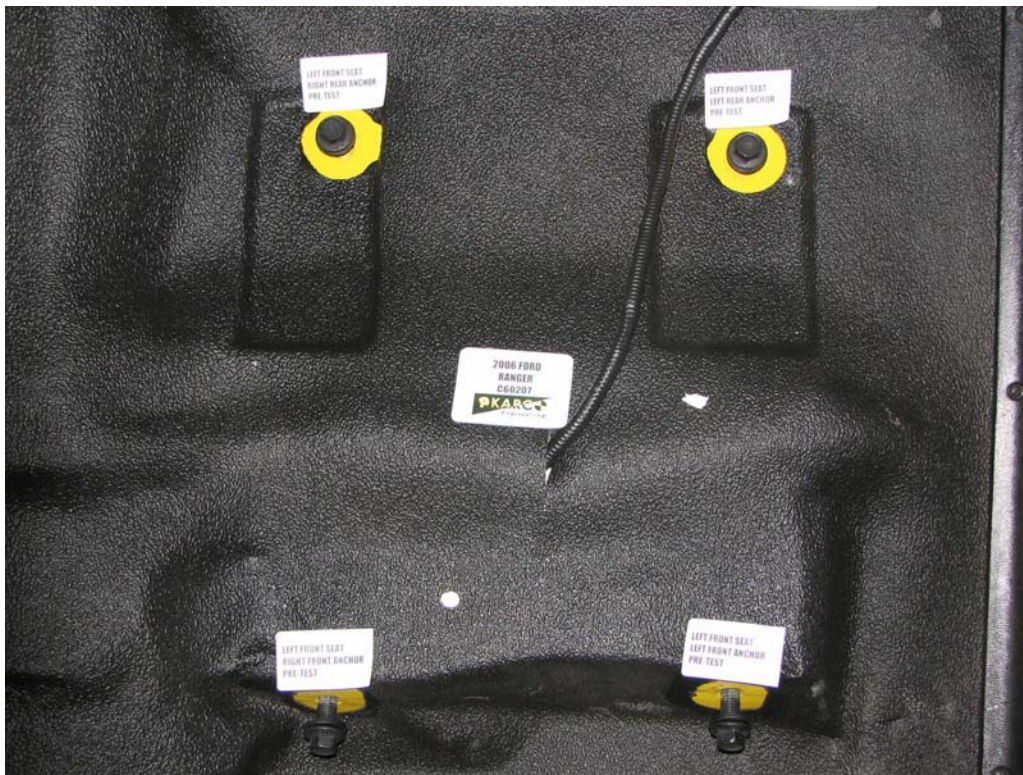
FIGURE 27. Floor Pan Anchors, P1 Overall, Pre-Test
