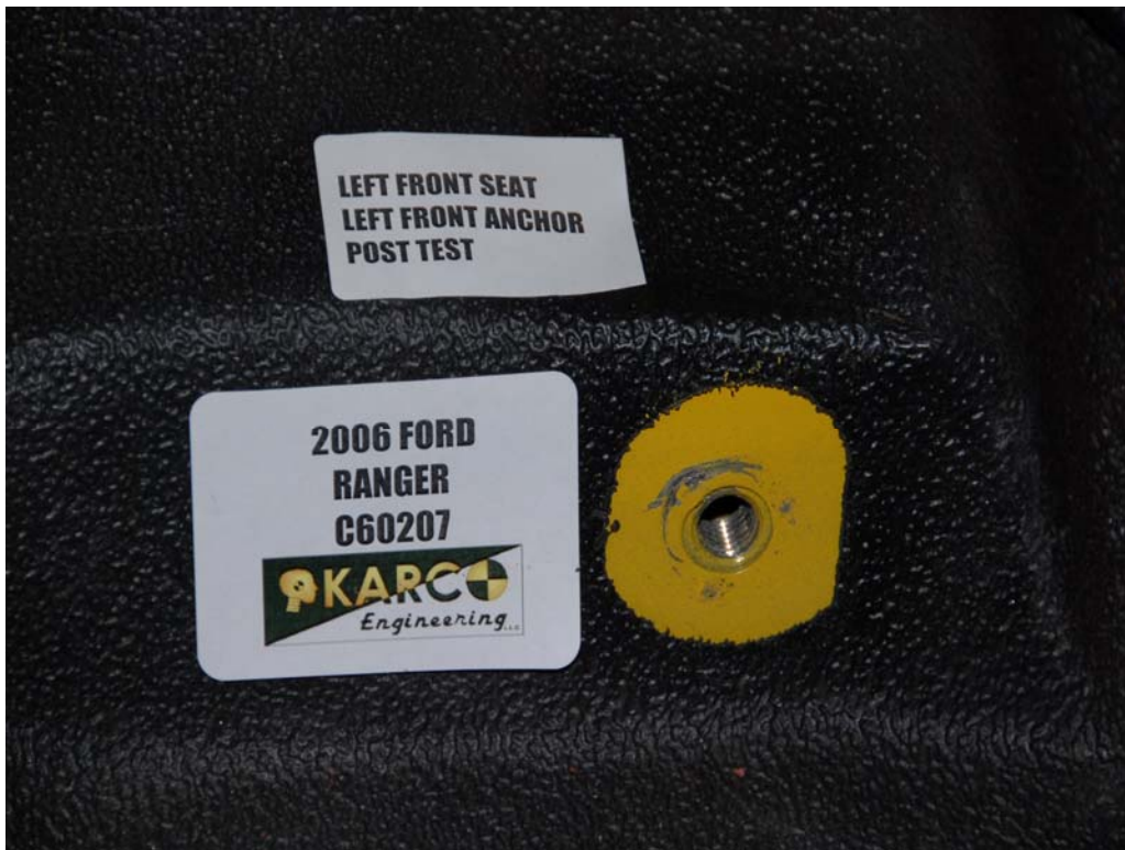
FIGURE 32. Floor Pan Anchor, P1, Post-Test
