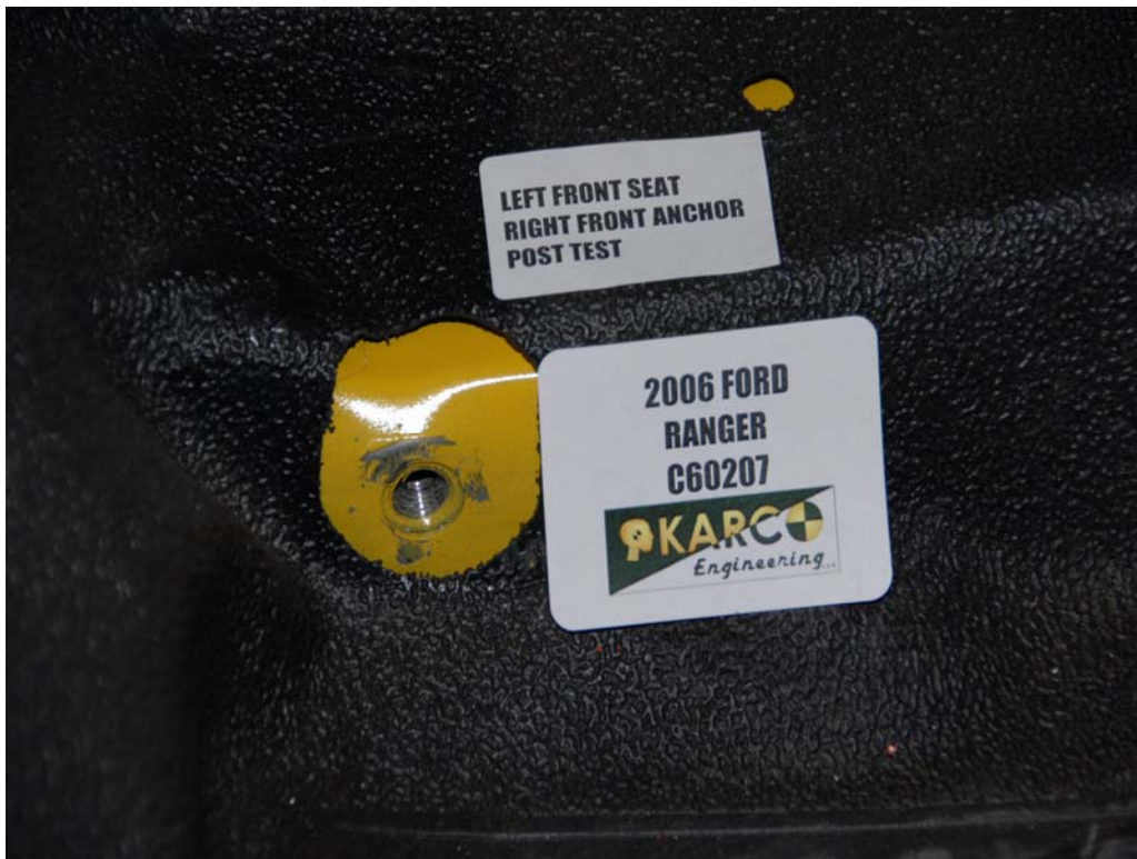
FIGURE 36. Floor Pan Anchor, P1, Post-Test
