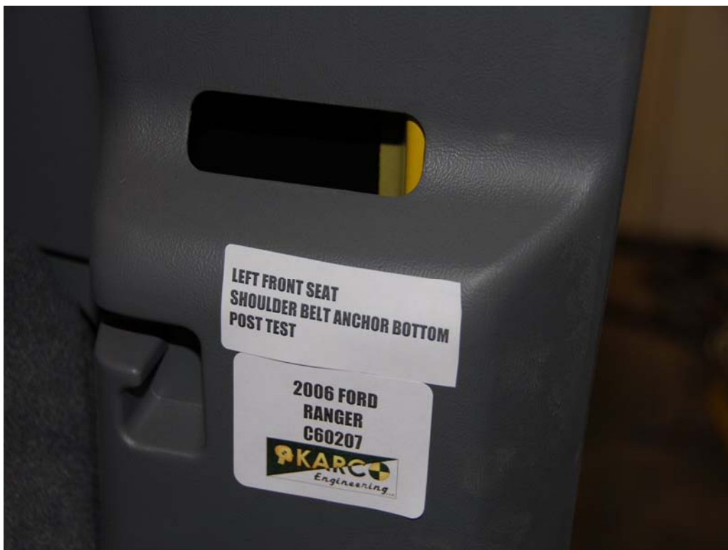
FIGURE 50. Shoulder Belt Anchor, P1, Post-Test
