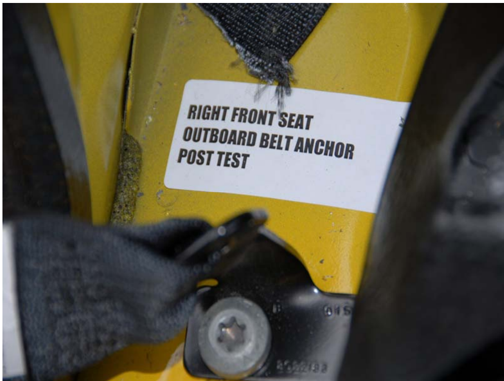
FIGURE 80. Belt Anchor, P2, Post-Test
