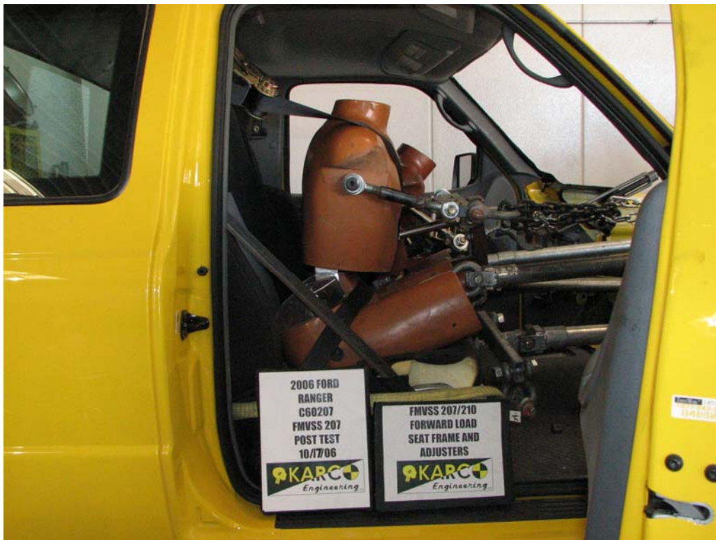
FIGURE 26. 207/210 Forward Load on Seat Frame and Adjusters, P2, Post-Test
