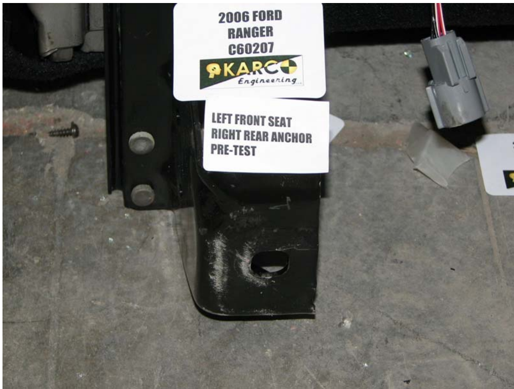
FIGURE 45. Seat Anchor, P1, Pre-Test
