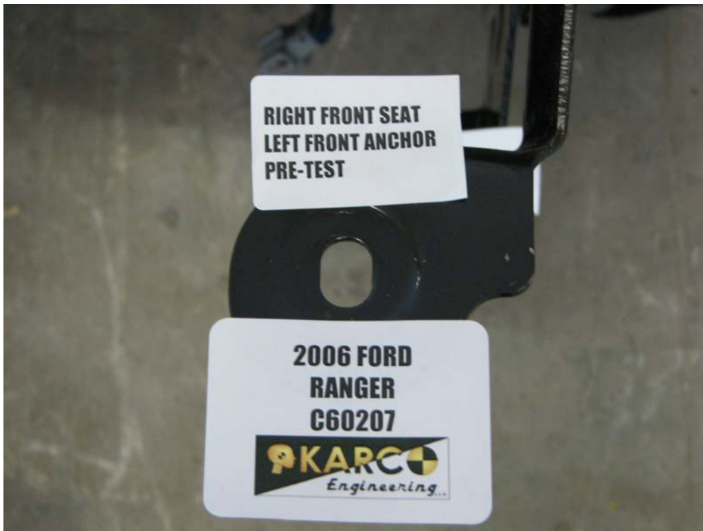
FIGURE 61. Seat Anchor, P2, Pre-Test
