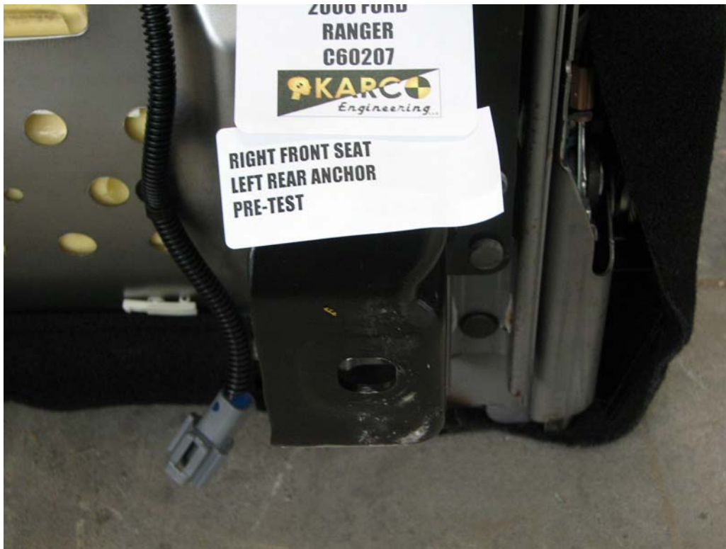
FIGURE 69. Seat Anchor, P2, Pre-Test
