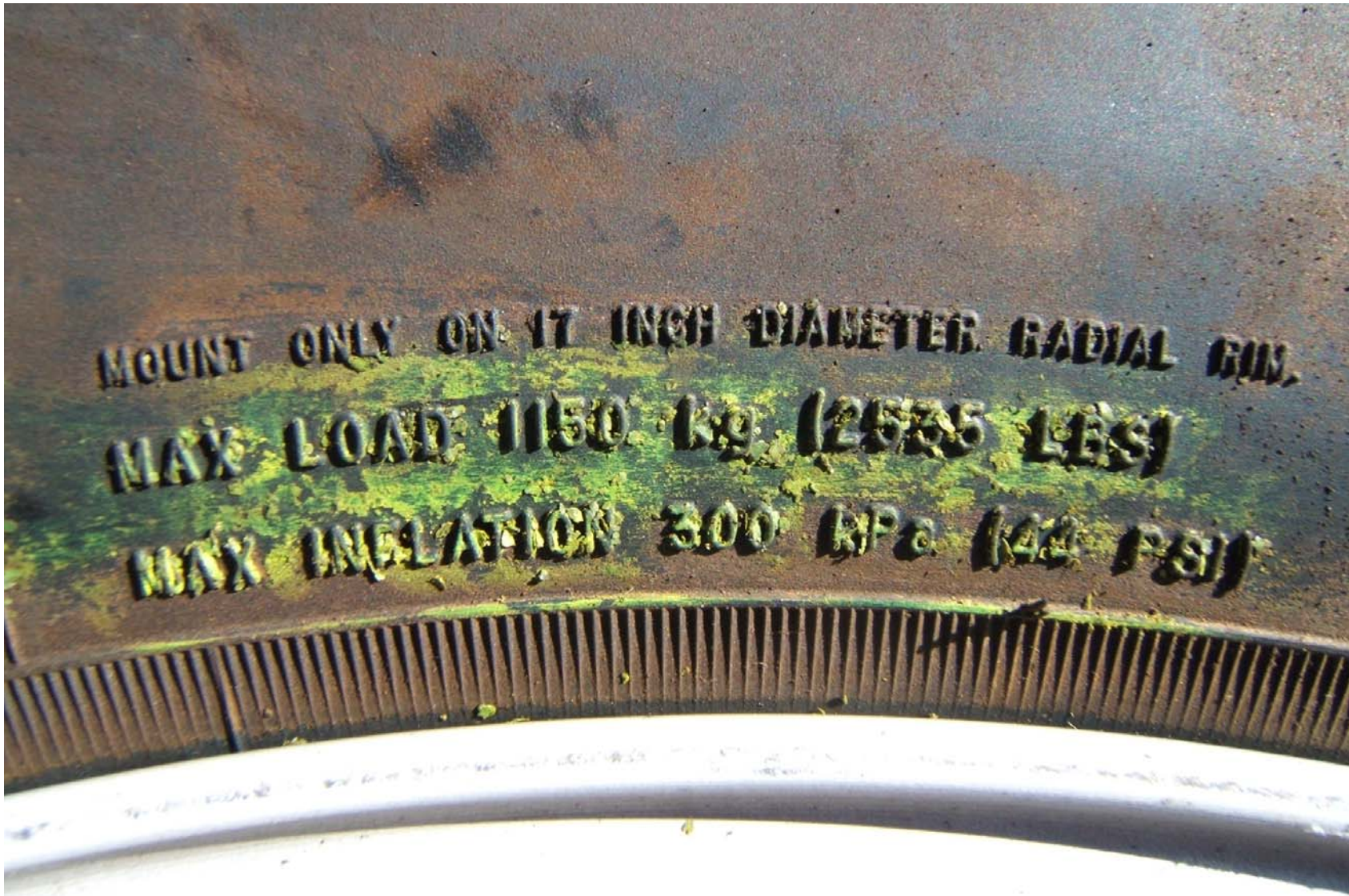
FIGURE 5.8 TIRE SHOWING MAX LOAD RATING AND MAX INFLATION PRESSURE
